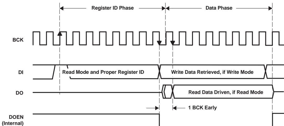
Figure 58. TDMCA Write and Read Operation Timing
