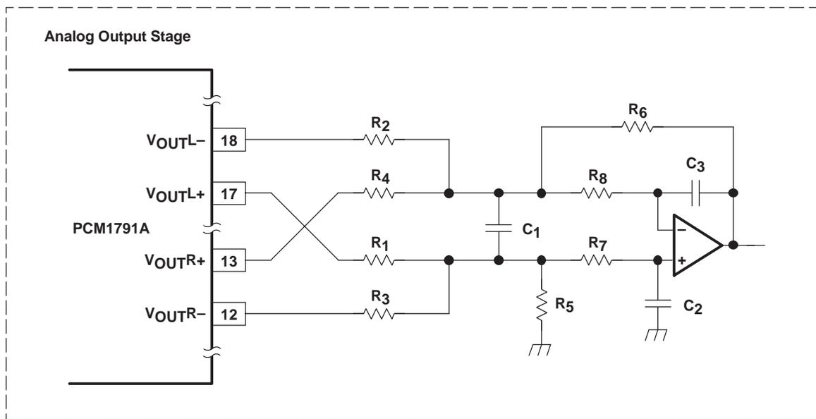
NOTE: Example R and C values for  $f_c = 77$  kHz, R1–R4: 3.6 k $\Omega$ , R5, R6: 3.3 k $\Omega$ , R7, R8: 680  $\Omega$ , C1: 1800 pF, C2, C3: 560 pF.
