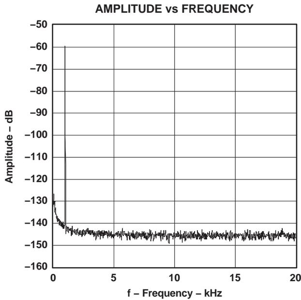
**Figure 19. -60-dB Output Spectrum, BW = 20 kHz**
