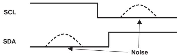
When these conditions occur at the same time, the PCM1791A erroneously detects a start or stop condition.
