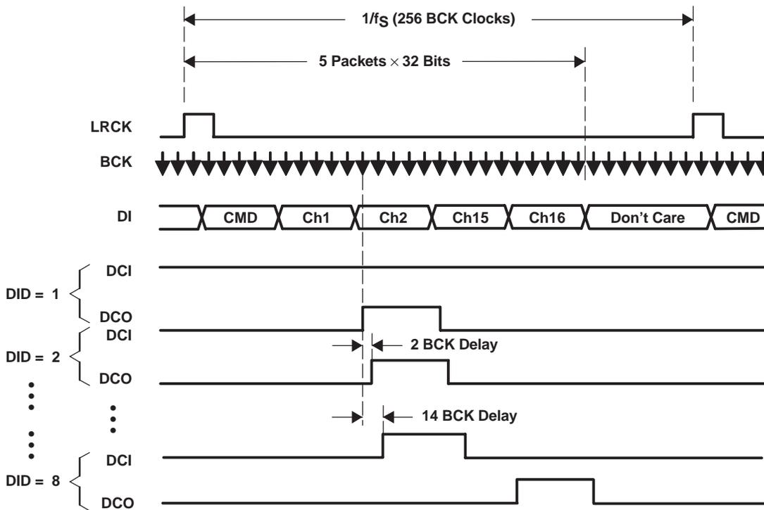
Figure 60. DCO Output Timing With Skip Operation
