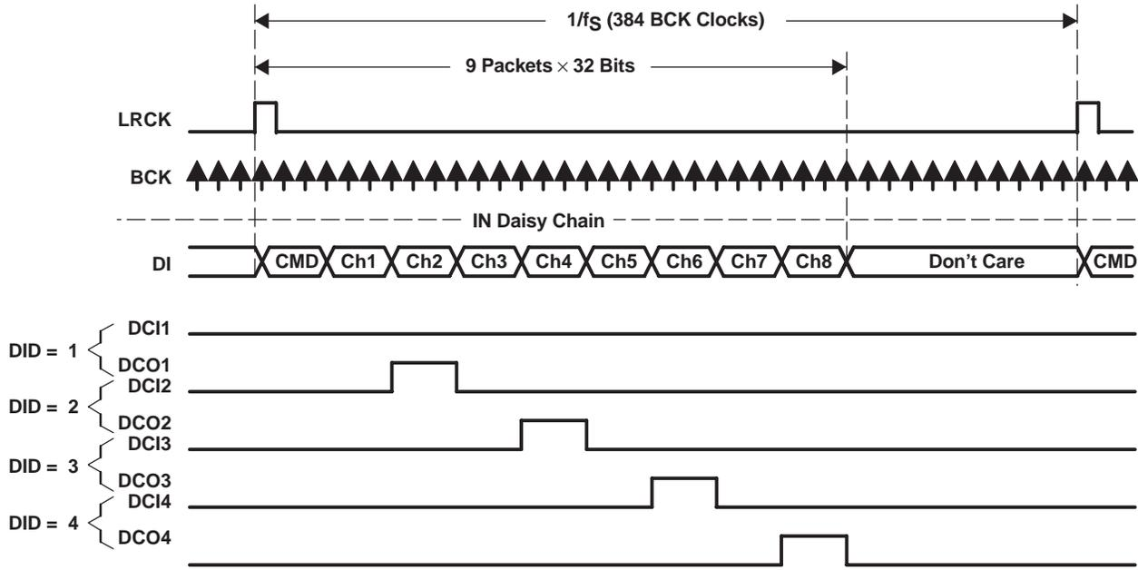
Figure 59. DCO Output Timing of TDMCA Mode Operation
