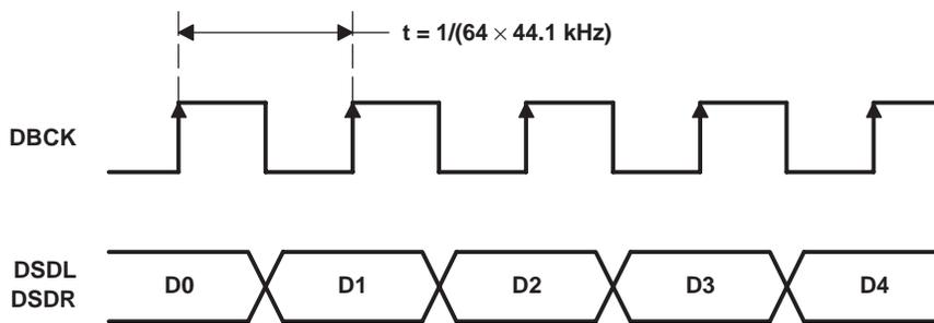
**Figure 42. Normal Data Output Form From DSD Decoder**
