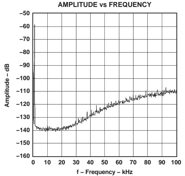
**Figure 20. -60-dB Output Spectrum, BW = 100 kHz**
