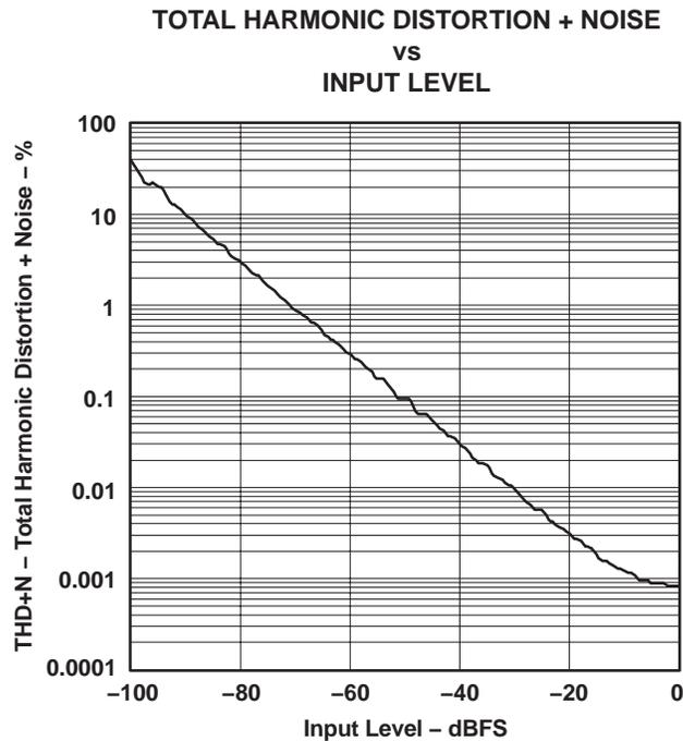
**Figure 21. THD+N vs Input Level, PCM Mode**
