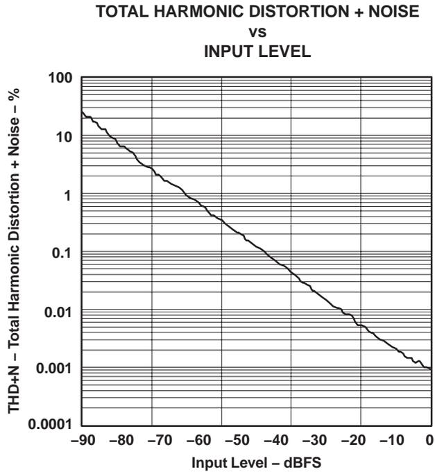
Figure 23. THD+N vs Input Level, DSD Mode
