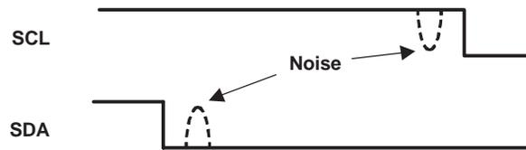
When these conditions occur at the same time, the PCM1791A fails to detect a start condition.
