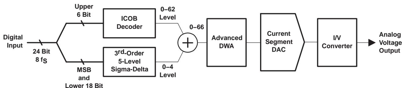
**Figure 63. Advanced Segment DAC With I/V Converter**
