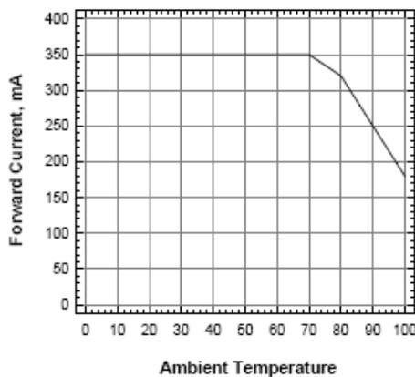
**Forward Current Vs Solder Point Temperature**
