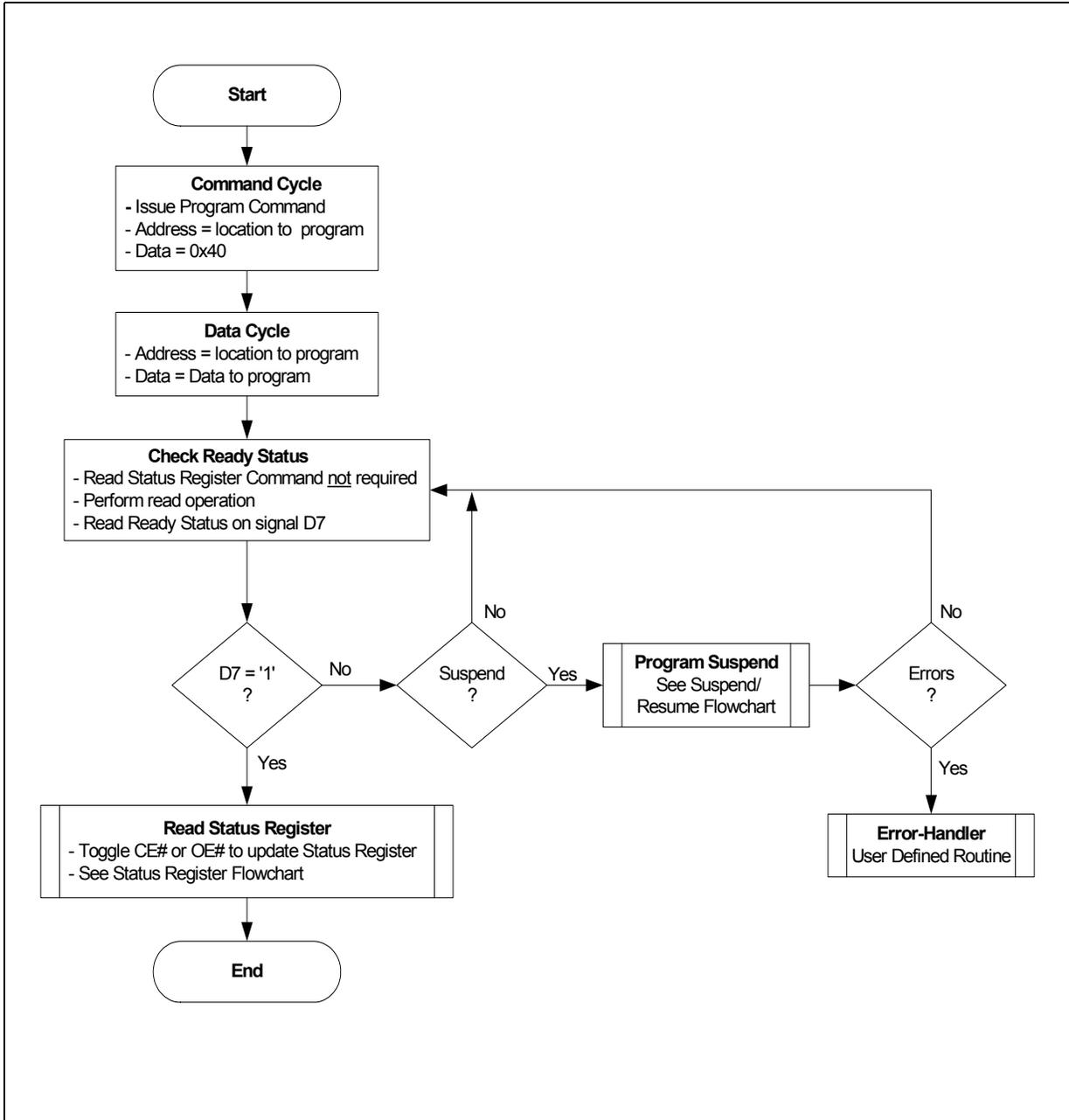
Figure 33: Program Suspend/Resume Flowchart
