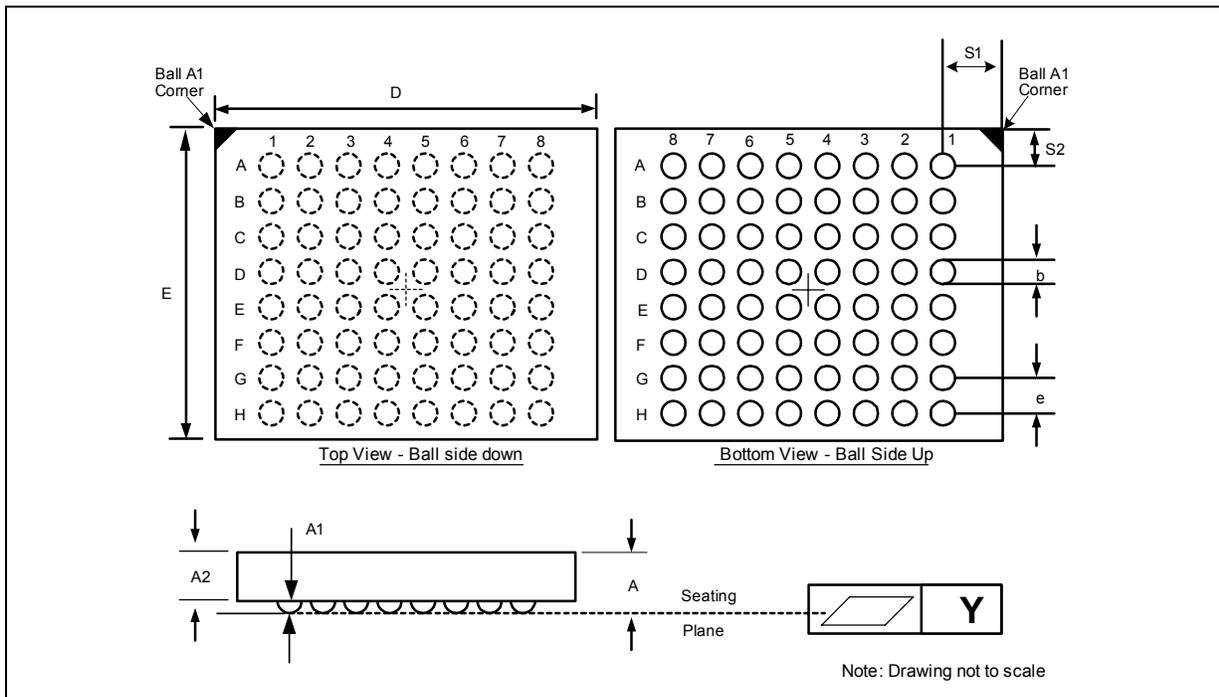
**Table 2: Easy BGA Package Dimensions for 10x13x1.2 mm (Sheet 1 of 2)**
