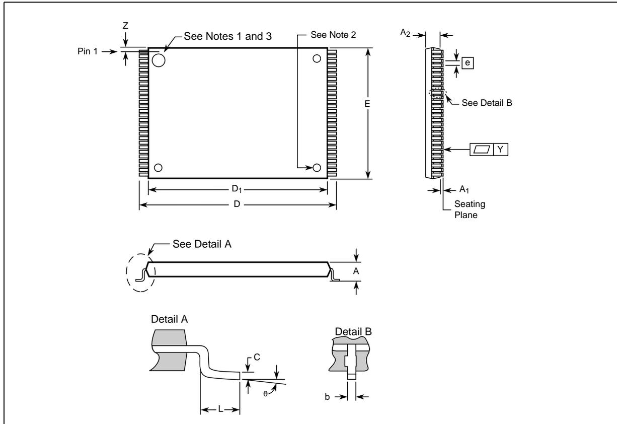
Table 1: TSOP Package Dimensions (Sheet 1 of 2)
