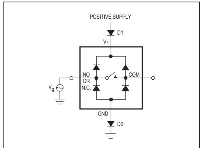
Figure 1. Overvoltage Protection Using Two External Blocking Diodes
