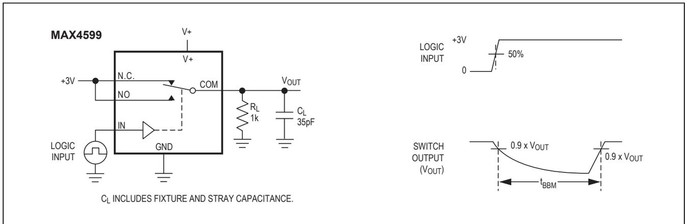
Figure 3. Break-Before-Make Interval
