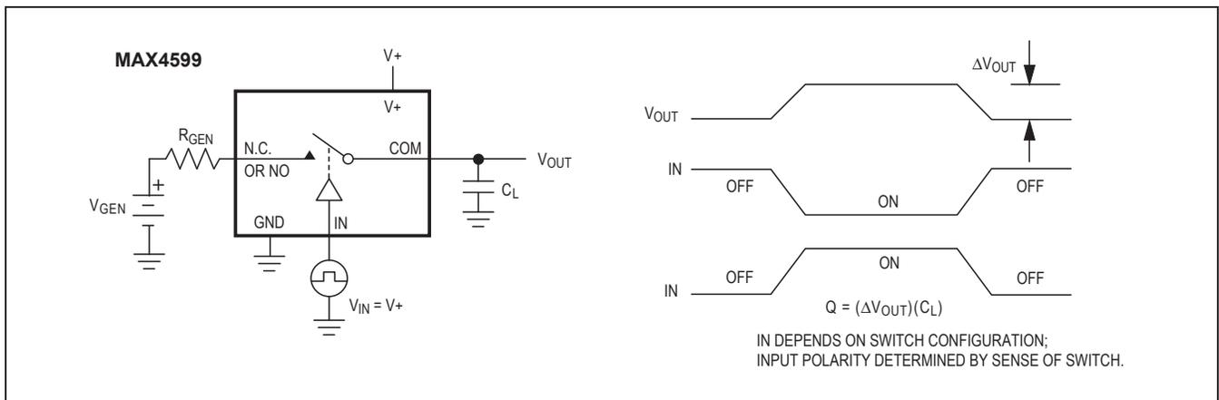
Figure 4. Charge Injection
