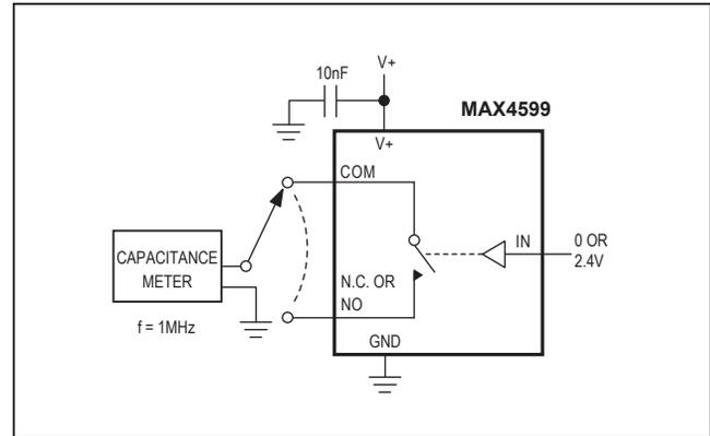
Figure 6. Channel On/Off-Capacitance
