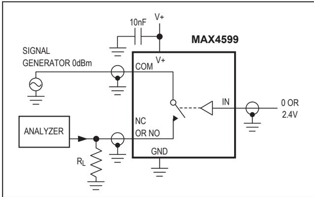
Figure 5. Off-Isolation/On-Channel Bandwidth
