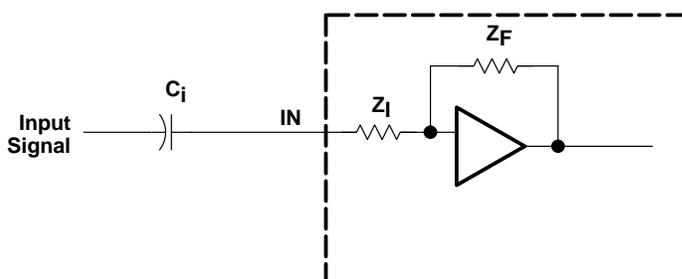
The -3 dB frequency can be calculated using equation 4.
