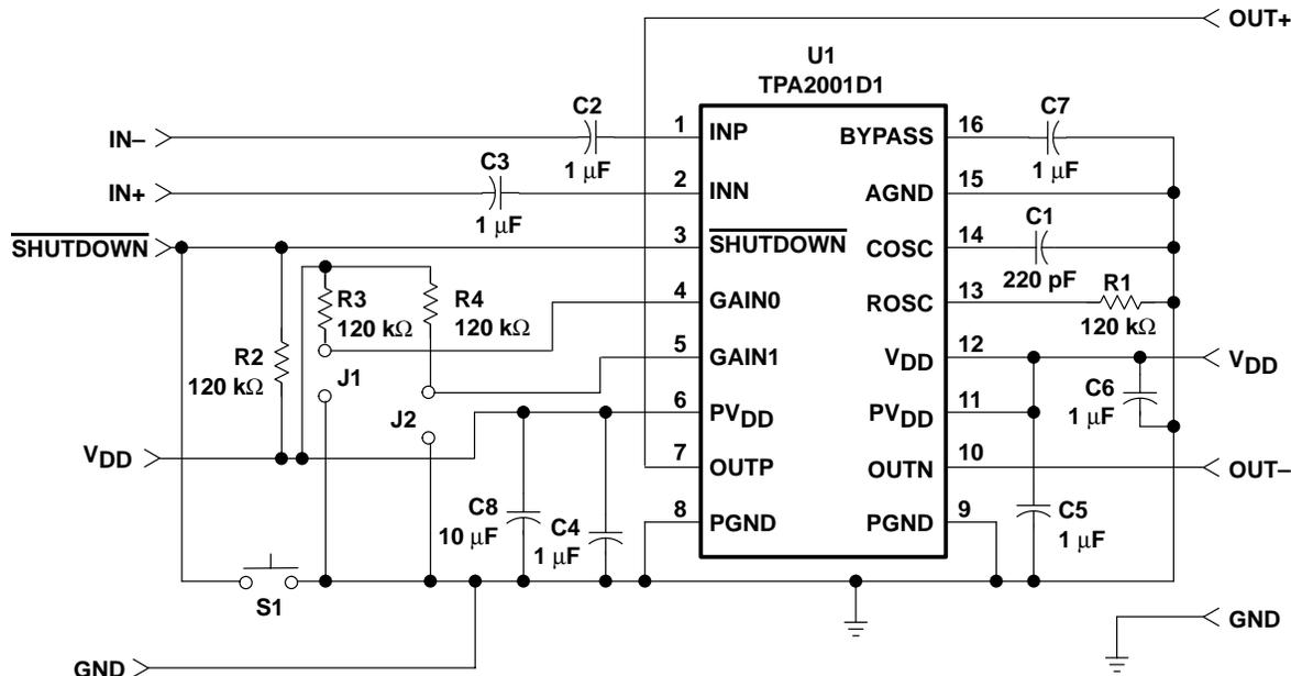
NOTE: R1, R2, and R3 are used in the EVM but are not required for normal applications.
