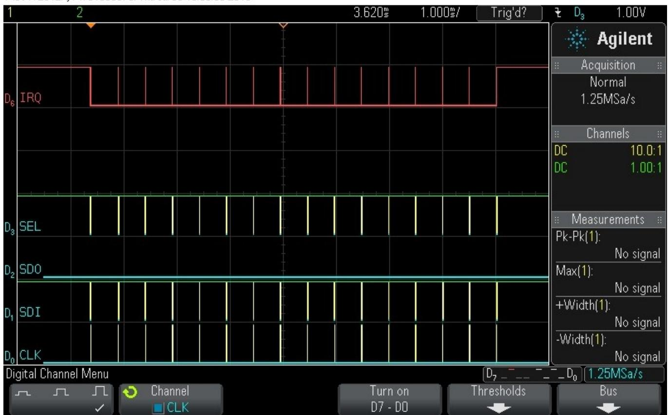
Above is the complete SPI & IRQ Timing diagram for #R<RSSI> <Packet >
