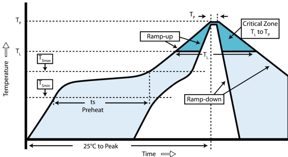
ZETA MODULE is a 2 layer PCB, re-flow is based on IPC/JEDEC JSTD020C July 2004
