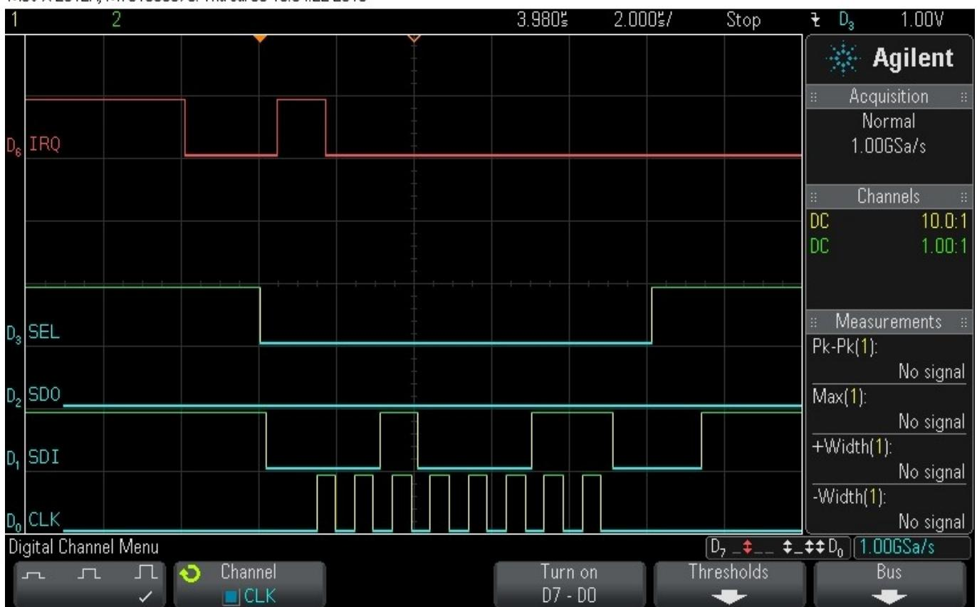
Above is the first byte of SPI data following U\_IRQ going low after an RF packet has been received.
