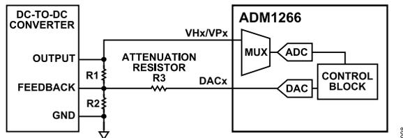
Figure 12. Typical Application Circuit for Margining
