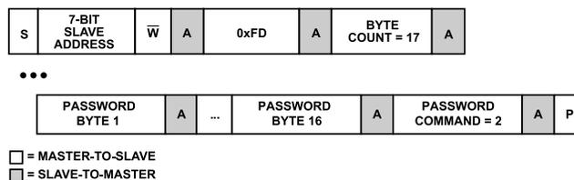
**Figure 16. Block Write Command for Unlocking the Device**
