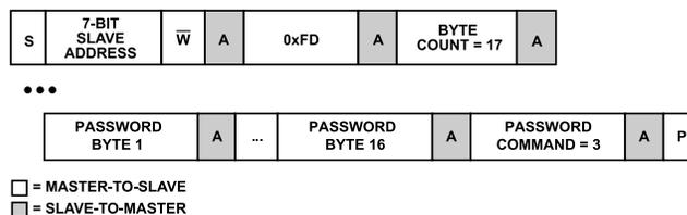
**Figure 17. Block Write Command for Locking the Device**
