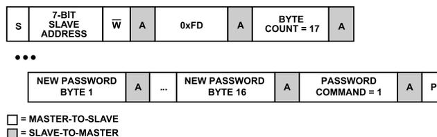
**Figure 18. Block Write Command for Changing the Password**
