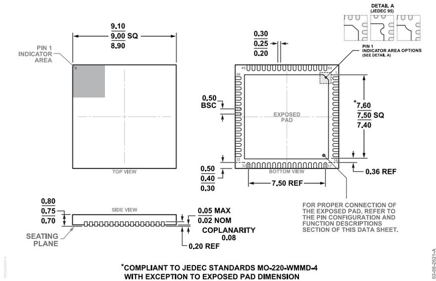
**Figure 30. 64-Lead Lead Frame Chip Scale Package [LFCS]
