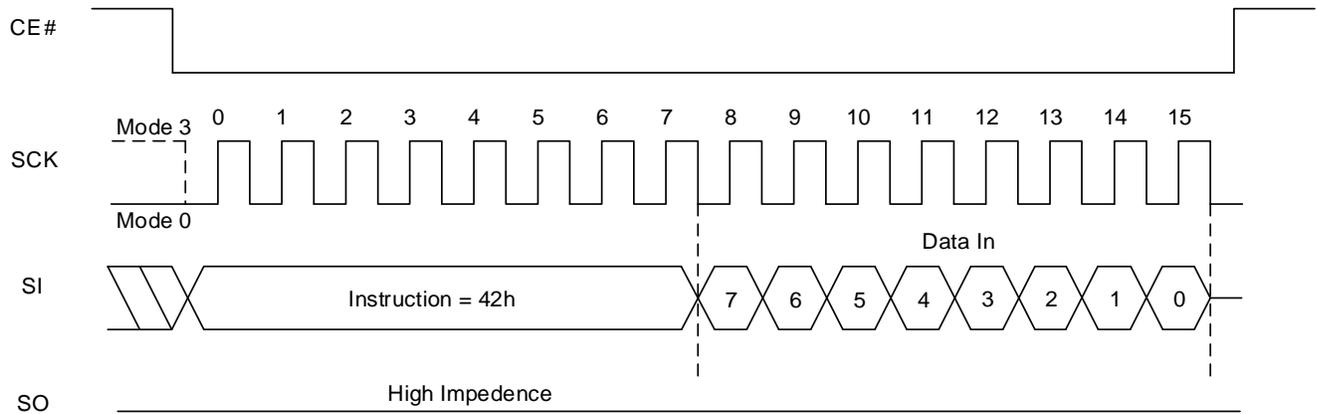
**Figure 8.33 Write Function Register QPI Sequence**
