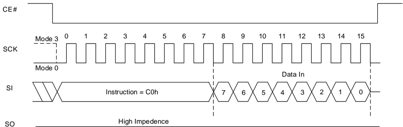
**Figure 8.41 Set Read Parameters QPI Sequence**
