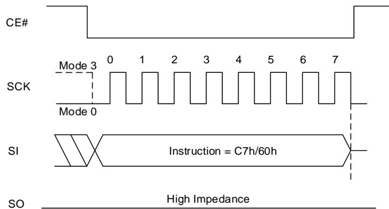
**Figure 8.21 Chip Erase QPI Sequence**
