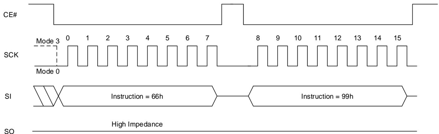
**Figure 8.51 Software Reset Enable and Software Reset QPI Sequence (RSTEN, 66h + RST, 99h)**
