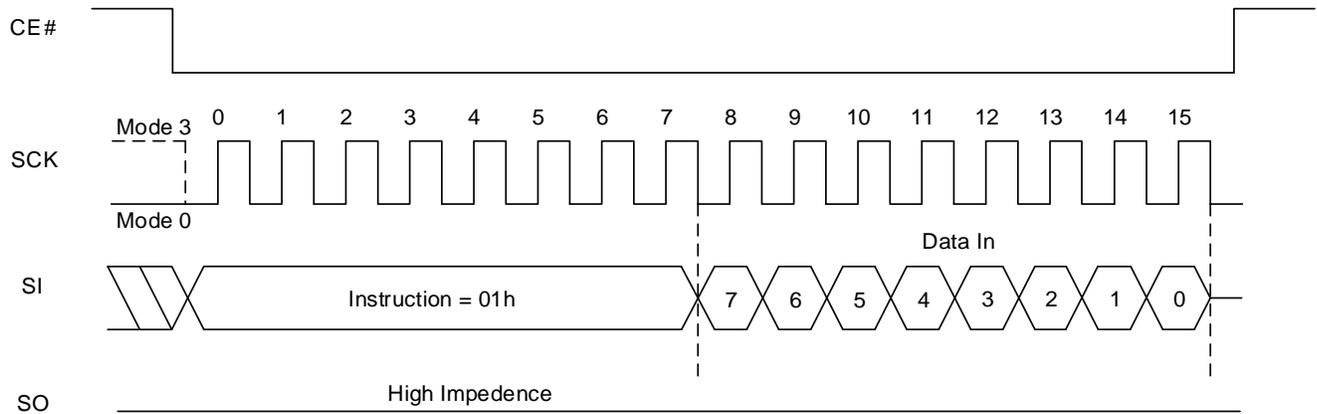
**Figure 8.29 Write Status Register QPI Sequence**
