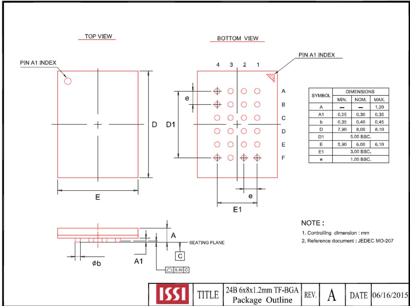
**10.6 24-BALL THIN PROFILE FINE PITCH BGA 6X8MM 5X5 BALL ARRAY (H)**
