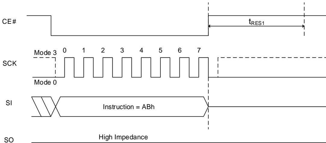
**Figure 8.39 Release Power Down QPI Sequence**
