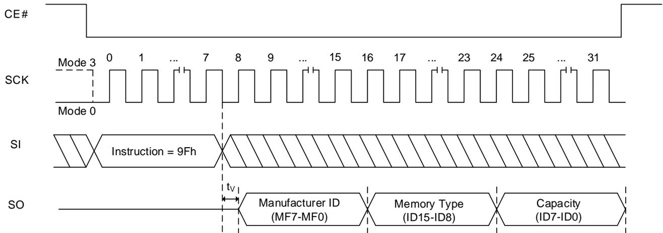
**Figure 8.45 RDJDID and RDJDIDQ (Read JEDEC ID) Sequence in QPI mode**
