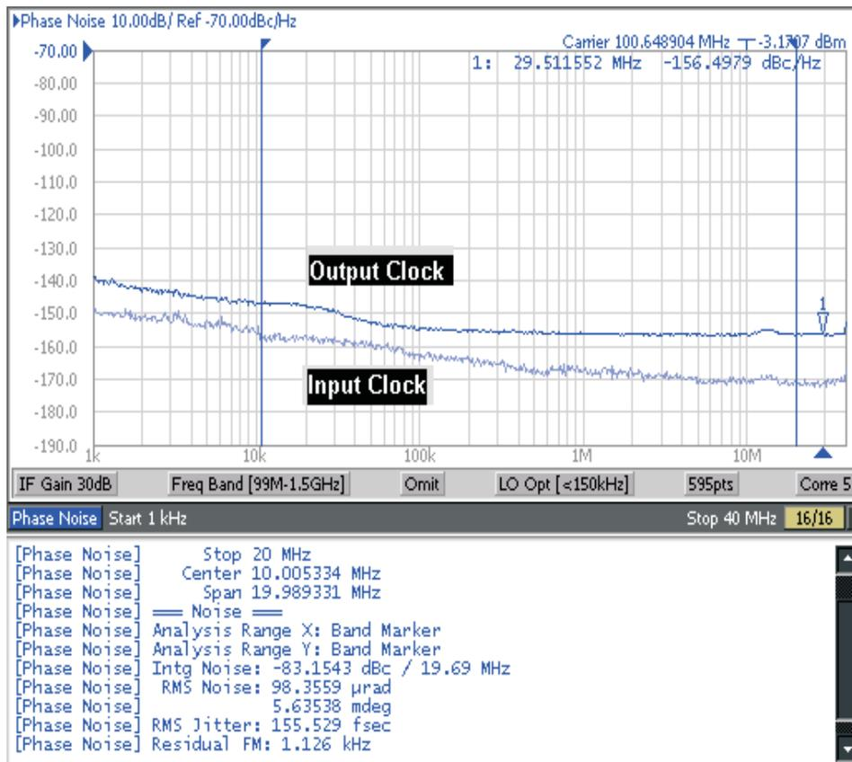
Input clock RMS jitter is 32 fs from 10 kHz to 20 MHz and additive RMS jitter is 152 fs
