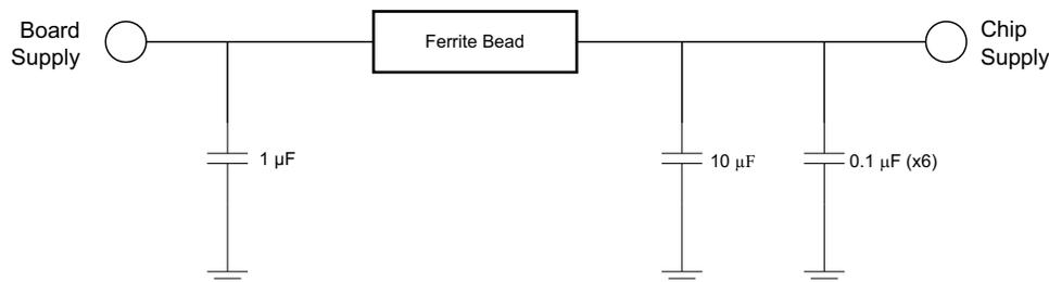
**Figure 12. Power-Supply Filtering**
