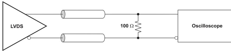
Figure 5. LVDS Output DC Configuration During Device Test
