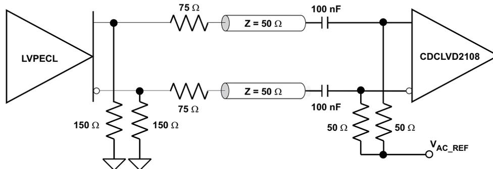
**Figure 17. LVPECL Clock Driver Connected to CDCLVD2108 Input**
