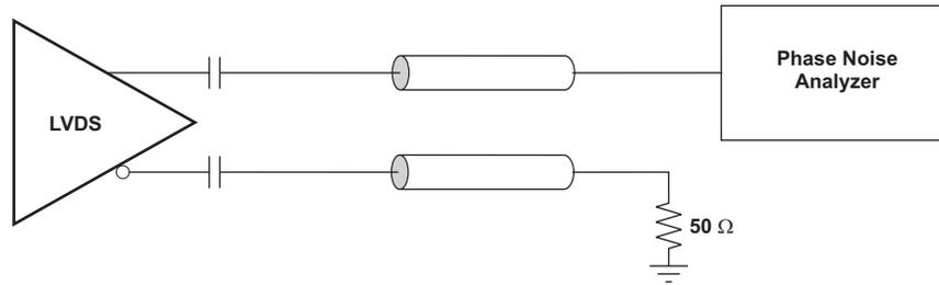
Figure 6. LVDS Output AC Configuration During Device Test
