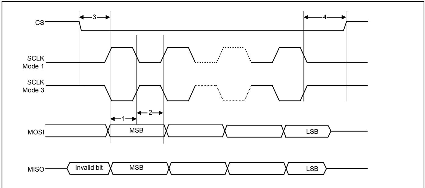
Table 20. SPI1 Timing Values—SCLK = 12 MHz and VDDM = 3.2V<sup>a</sup>
