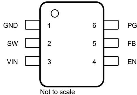
**Figure 6-1. 6-Pin DRL SOT-563 Package (Top View)**
