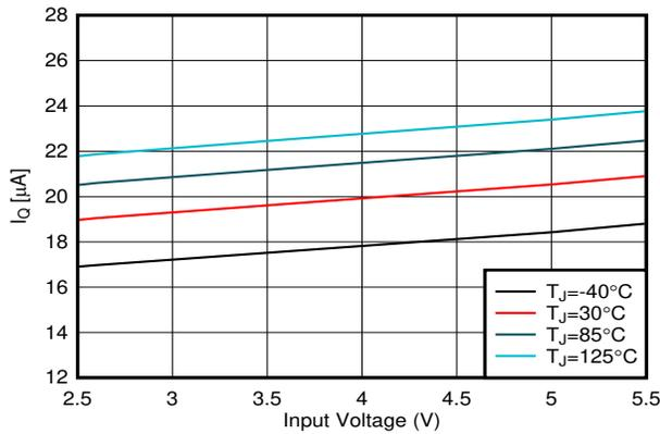
**Figure 7-1. Quiescent Current vs Input Voltage (TPS62A01)**
