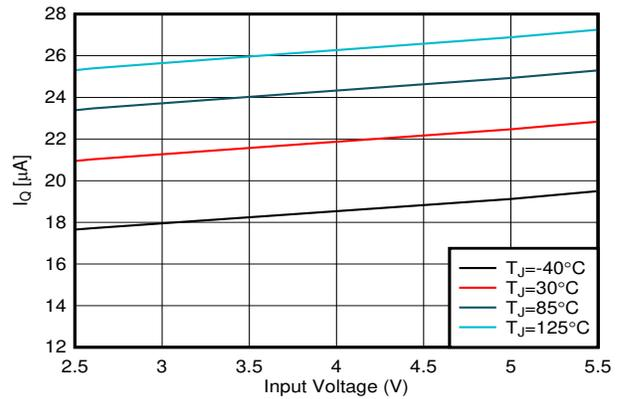
**Figure 7-2. Quiescent Current vs Input Voltage (TPS62A02)**
