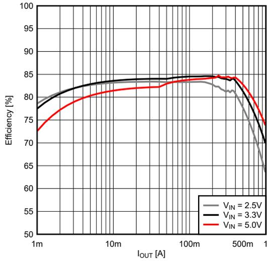
Figure 9-3. 0.6-V Output Efficiency (TPS62A01)
