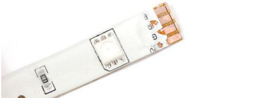
Melt some solder onto the pads to tin them and also burn away any left over rubber.
