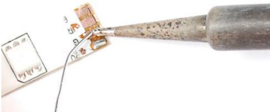
Solder the four wires on. We used stranded wire, which is more flexible and is probably a better choice than solid-core.
