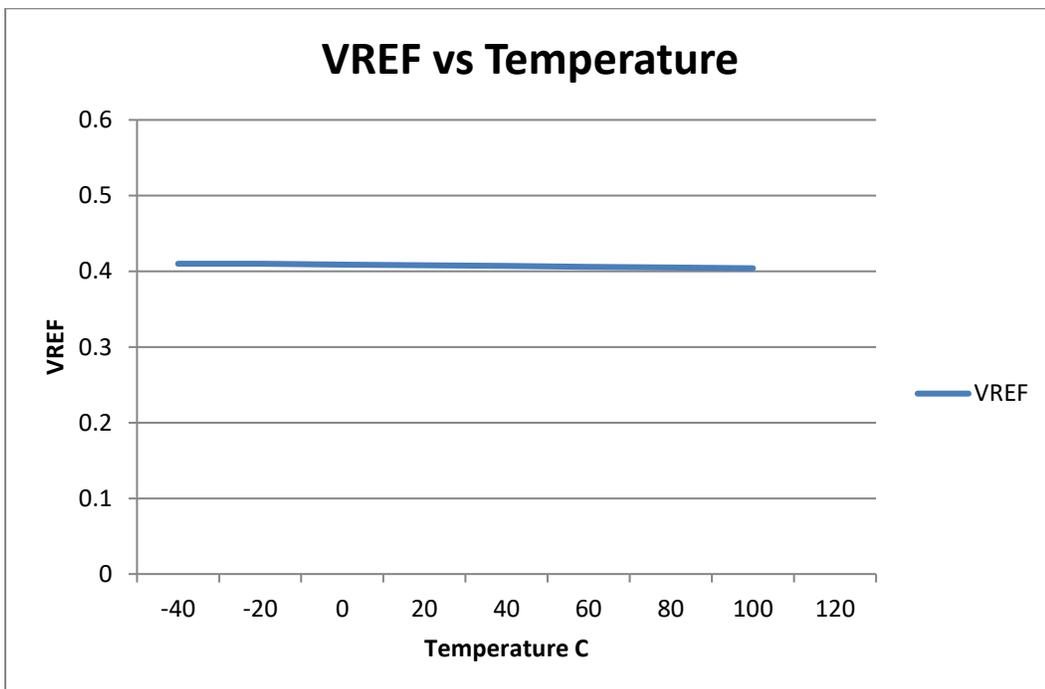
Figure 14: Feedback voltage reference (VFB) over temperature
