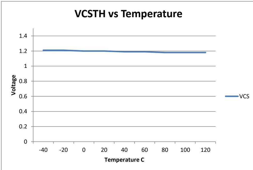
Figure 13: Over current threshold (VCSTH) over temperature
