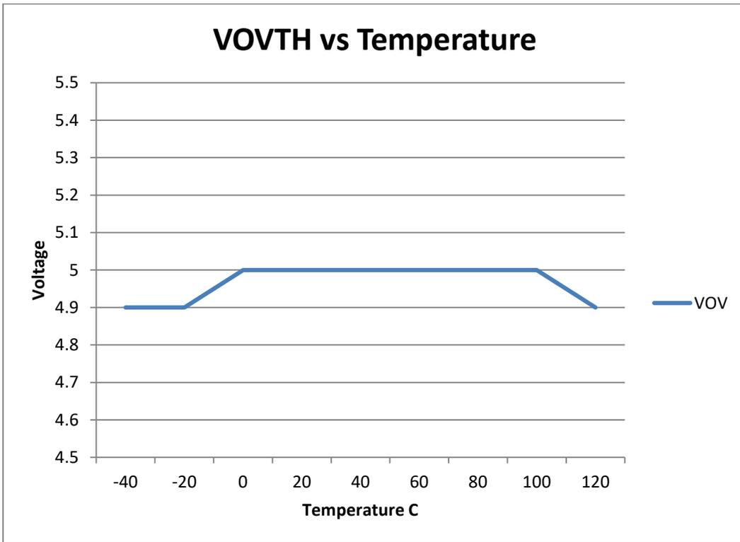
Figure 12: Over voltage threshold (VOVTH) over temperature
