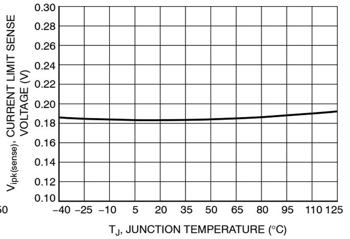
**Figure 12. Current Limit Sense Voltage vs. Temperature**
