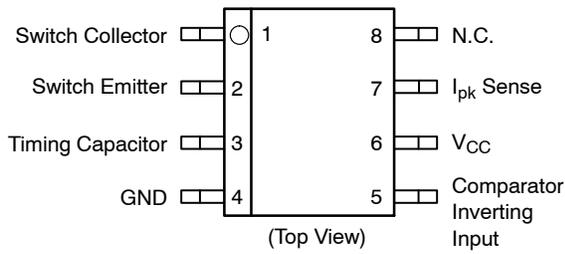
Figure 2. Pin Connections
