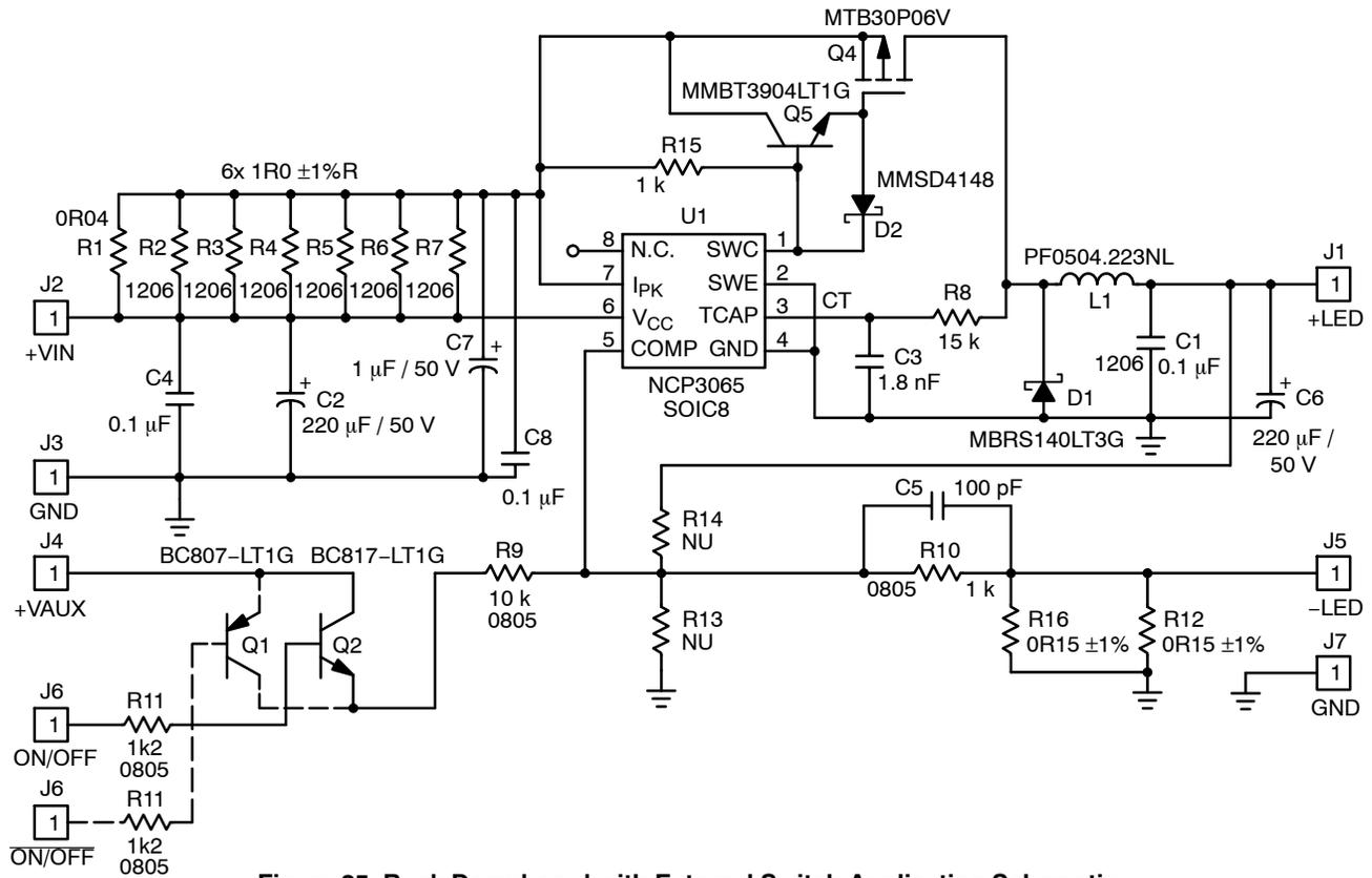
**Figure 25. Buck Demoboard with External Switch Application Schematic**
