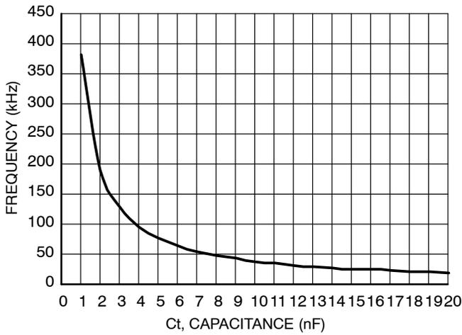
**Figure 5. Oscillator Frequency vs. Oscillator Timing Capacitor**
