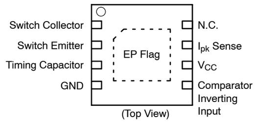
Figure 3. Pin Connections
