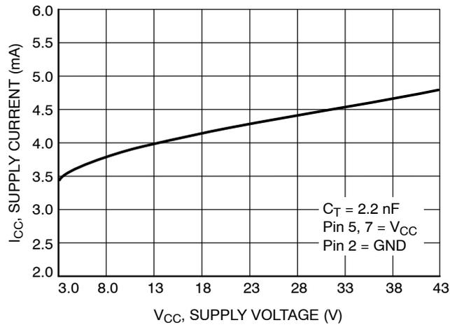
**Figure 13. Standby Supply Current vs. Supply Voltage**
