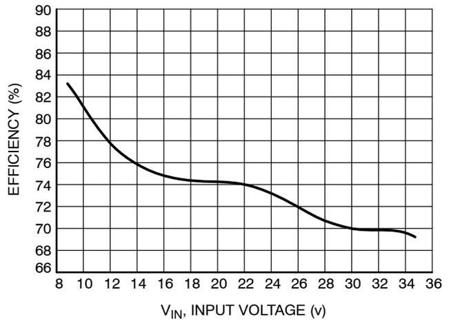
Figure 27. Efficiency vs. Input Voltage for the 3 A Buck Demo Board at I<sub>OUT</sub> = 3 A, V<sub>OUT</sub> = 4 V, T<sub>A</sub> = 25°C
