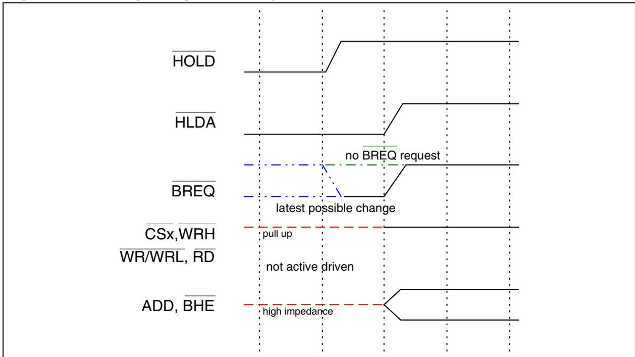
Note: The falling  $\overline{BREQ}$  edge shows the last chance for  $\overline{BREQ}$  to trigger the indicated regain-sequence. Even if  $\overline{BREQ}$  is activated earlier the regain-sequence is initiated by  $\overline{HOLD}$  going high. Please note that  $\overline{HOLD}$  may also be deactivated without the C166S V2 requesting the bus.
