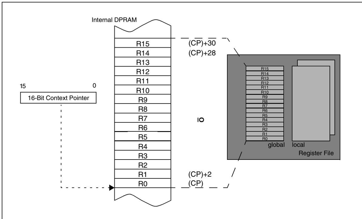
**Figure 2-9 Register Bank Selection via Register CP**
