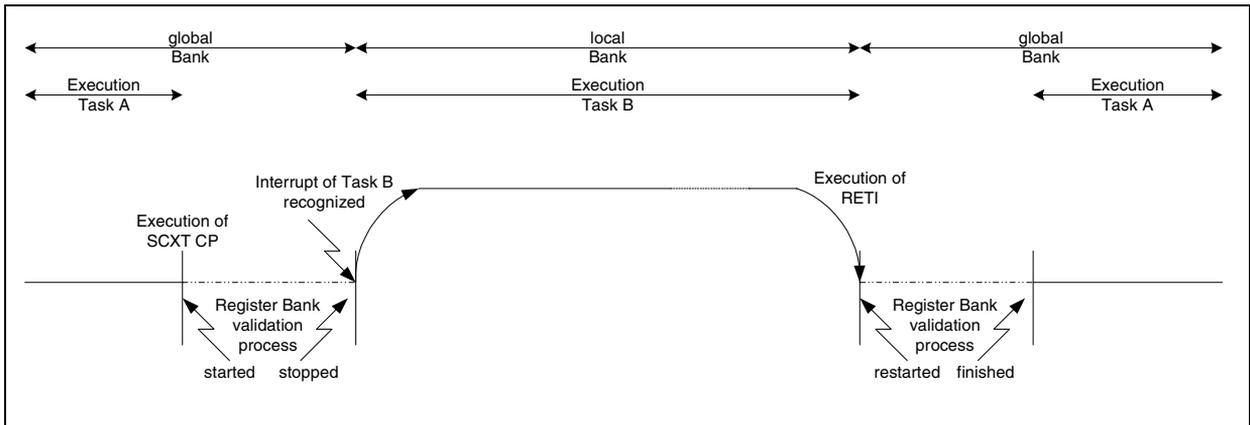
**Note: Validation Process and Hardware Interrupts using a Local Register Bank**
