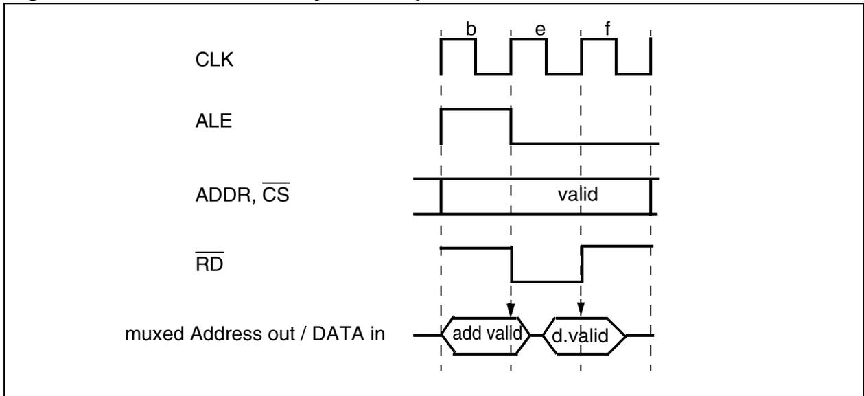
**Figure 6-14 Fastest Write Cycle Multiplexed Bus**
