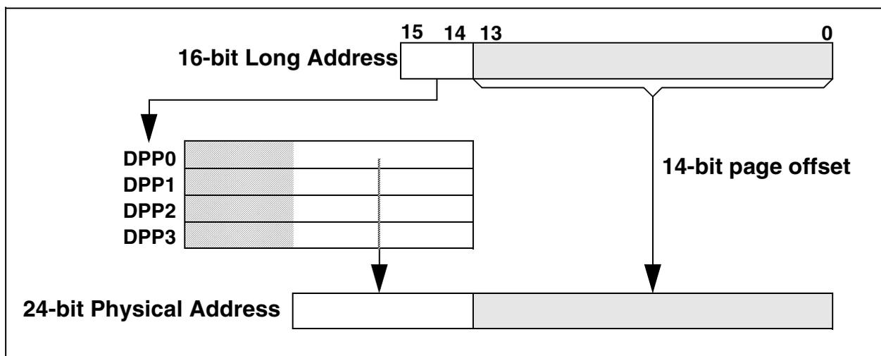
**Figure 2-14 Interpretation of a 16-bit Long Address**
