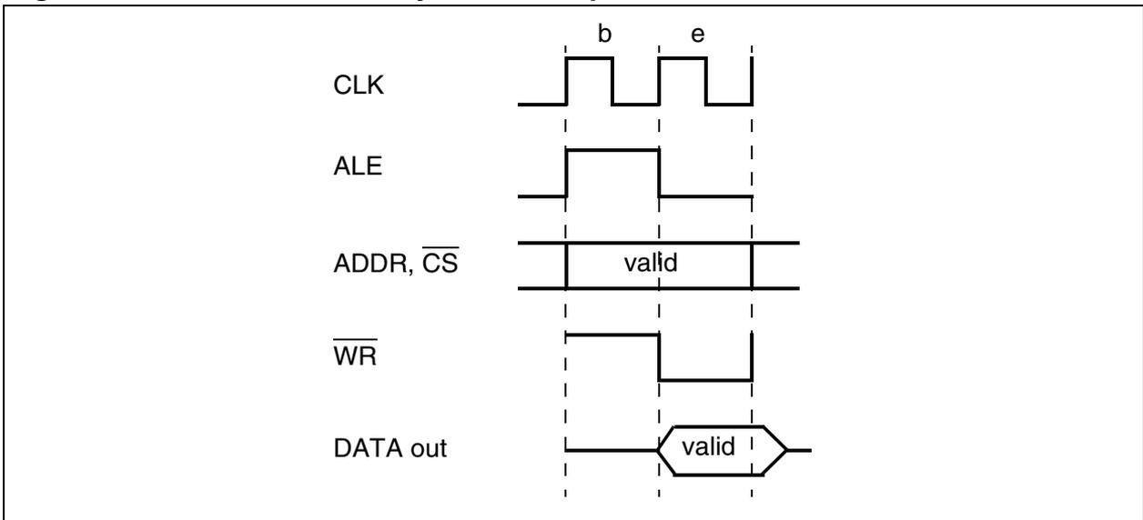
**Figure 6-13 Fastest Read Cycle Multiplexed Bus**
