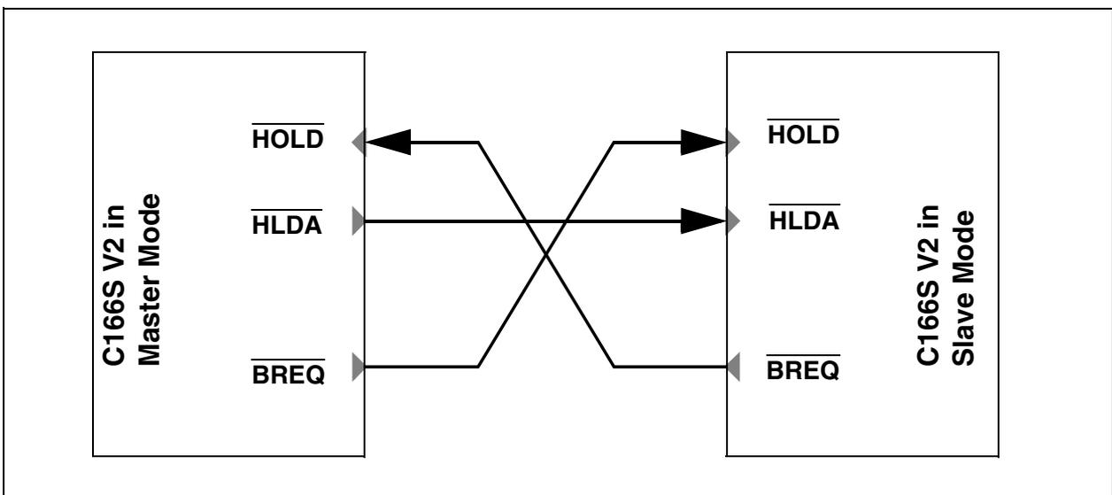
**Figure 6-10 Connecting two C166S V2s using Master/Slave Arbitration**
