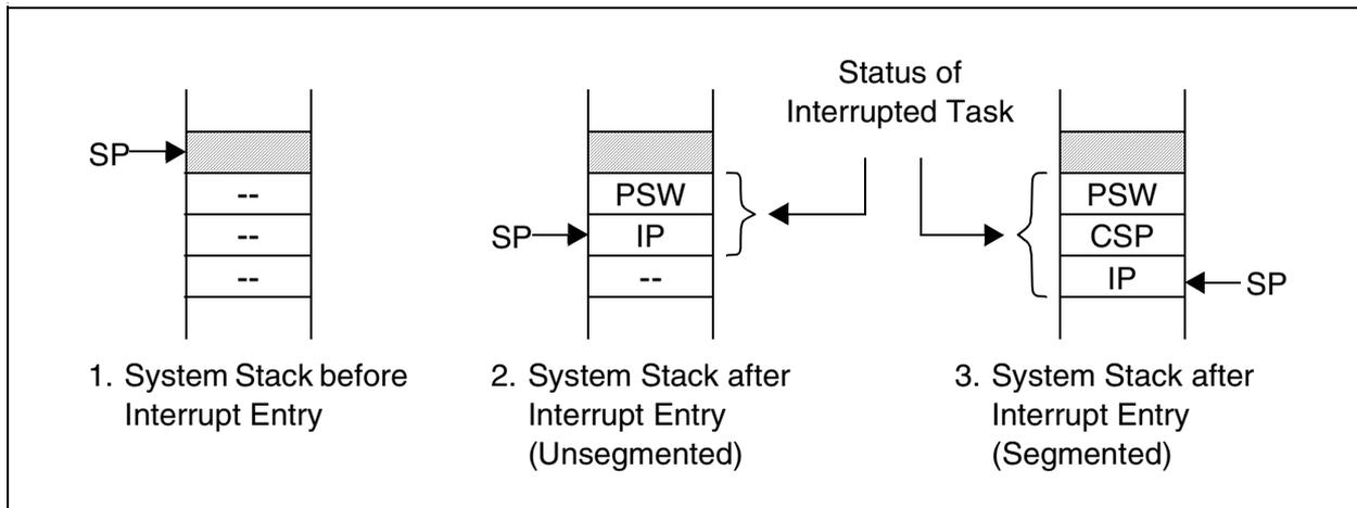
**Figure 5-3 Task Status Saved on the System Stack**
