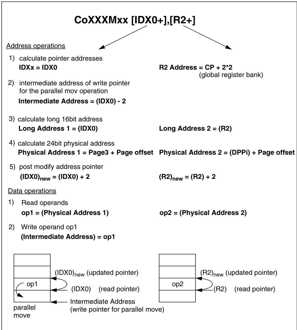
**Figure 2-19 Arithmetic MAC Operations with Parallel Move**
