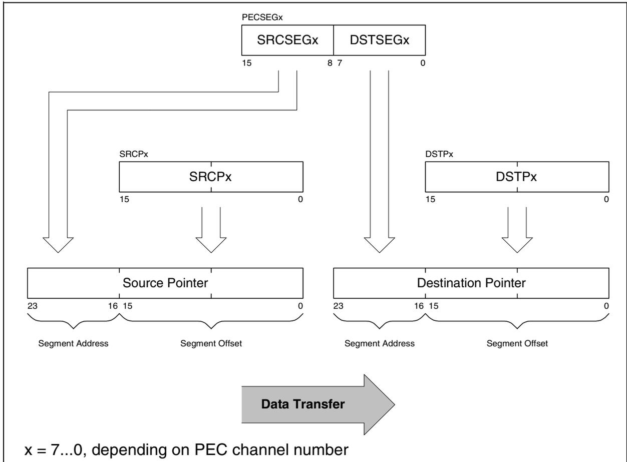
**Figure 5-5 PEC Pointer Address Handling**
