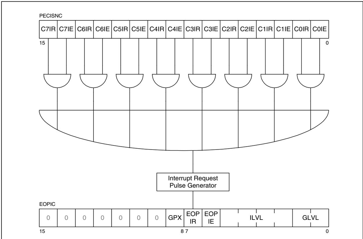
**Figure 5-4 End of PEC Interrupt Sub Node**
