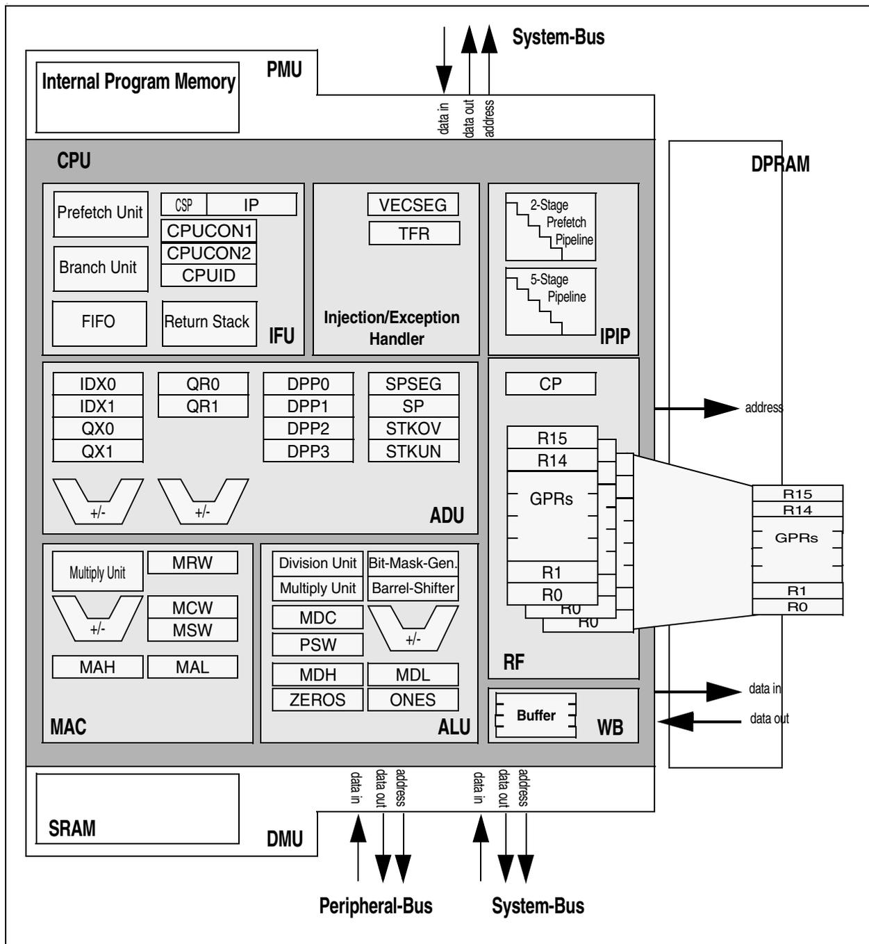
Figure 2-1 CPU Architecture
