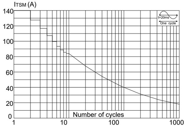
**FIG.5:** Non-repetitive surge peak on-state current for a sinusoidal pulse with width  $t_p < 20ms$  and corresponding value of  $f \cdot t$  (I - II - III:  $di/dt < 50A/\mu s$ ; IV:  $di/dt < 10A/\mu s$ )
