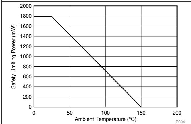
Figure 3. Thermal Derating Curve for Limiting Power per VDE for DW-16 Package
