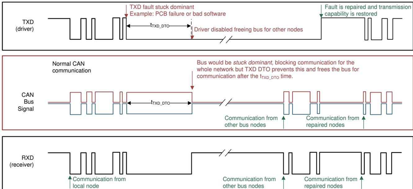
Figure 27. Example Timing Diagram for TXD DTO
