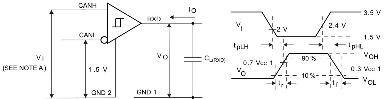
A. The input pulse is supplied by a generator having the following characteristics: PRR ≤ 125 kHz, 50% duty cycle,  $t_r \leq 6$  ns,  $t_f \leq 6$  ns,  $Z_O = 50 \Omega$ .
