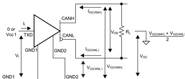
Figure 15. Driver Voltage, Current and Test Definitions
