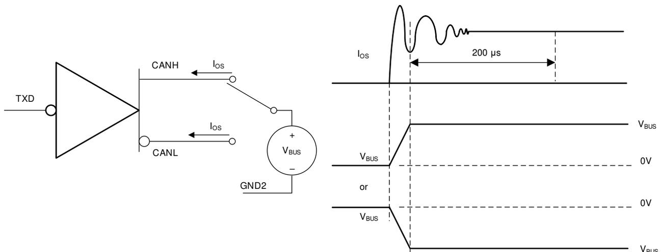
Figure 23. Driver Short-Circuit Current Test Circuit and Waveforms
