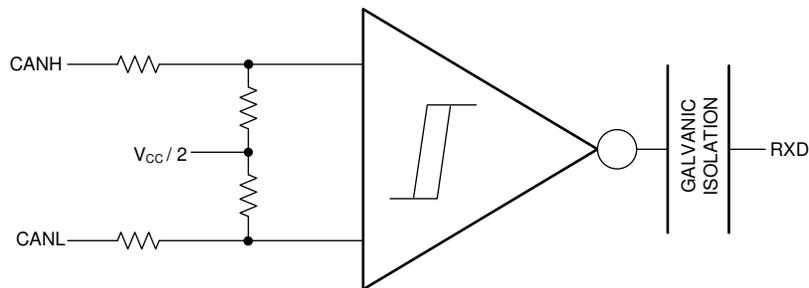
**Figure 26. Simplified Recessive Common Mode Bias and Receiver**
