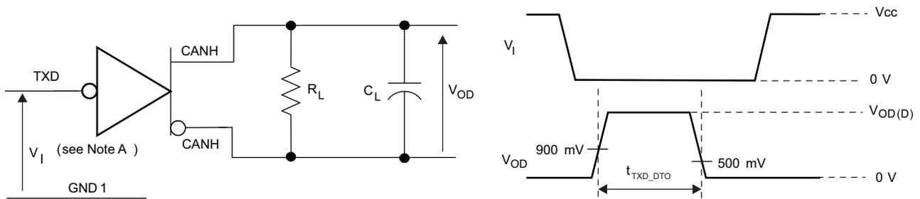
A. The input pulse is supplied by a generator having the following characteristics:  $t_r \leq 6$  ns,  $t_f \leq 6$  ns,  $Z_O = 50 \Omega$ .
