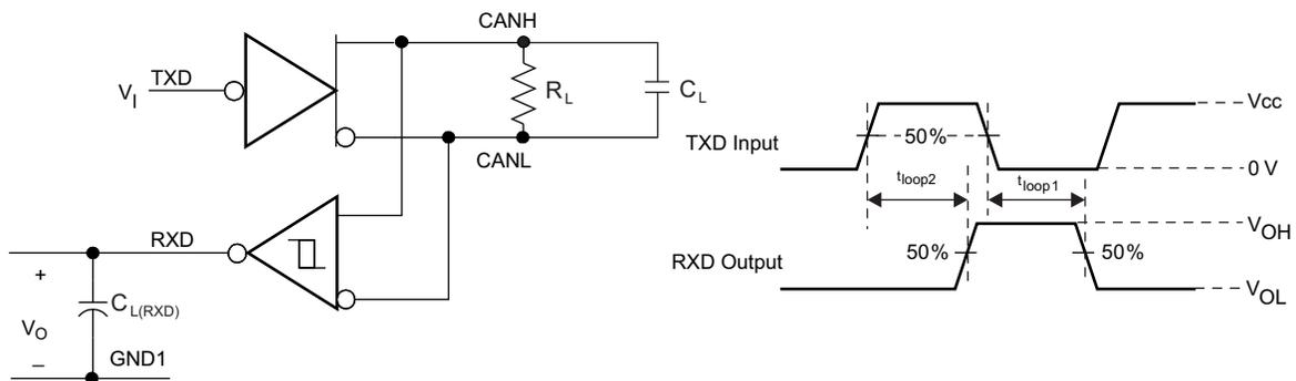
Figure 20.  $t_{LOOP}$  Test Circuit and Voltage Waveforms
