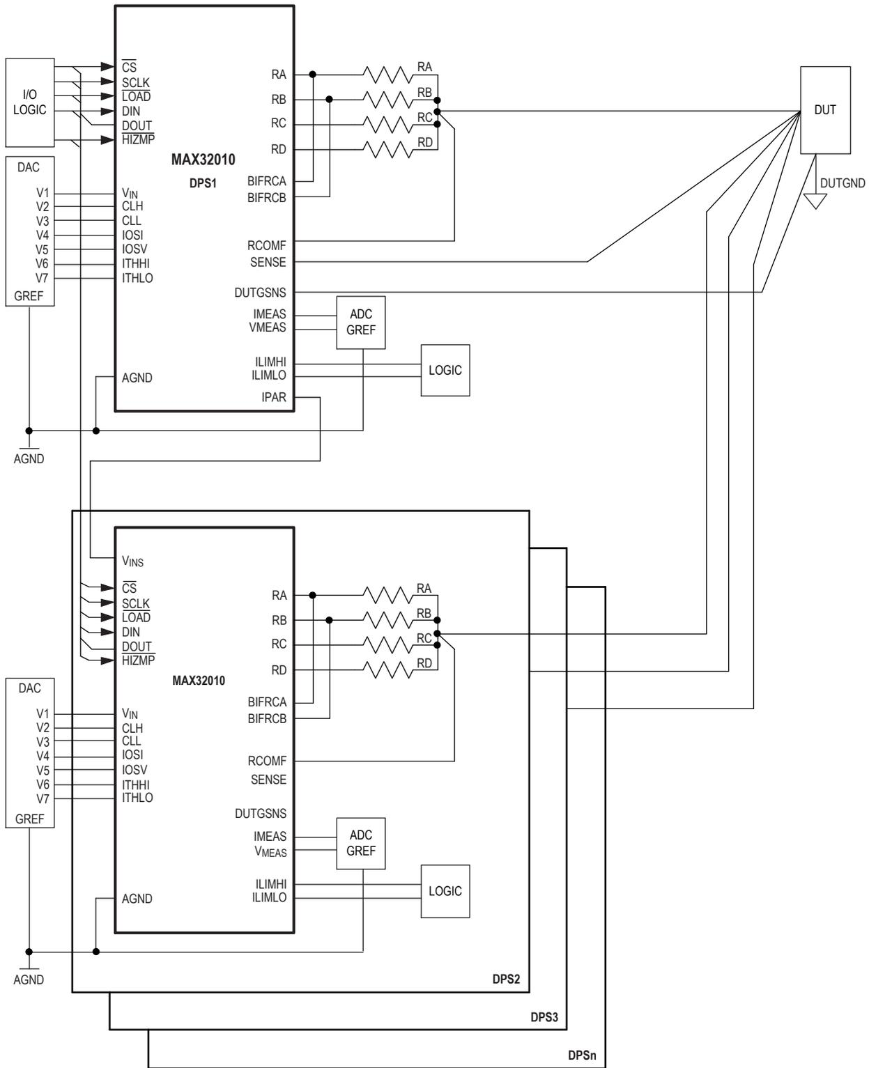
Figure 7. Parallel DPS Configuration Achieves Higher Output Current
