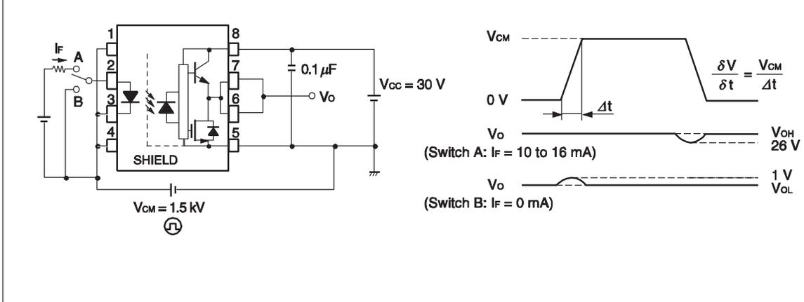
**Remark** CMR Test : Connect pin 1 and pin 4 to the LED common.
