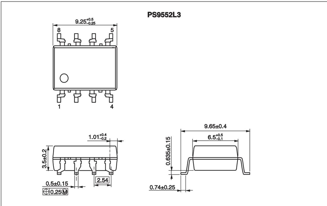
Lead Bending Type For Long Creepage Distance
