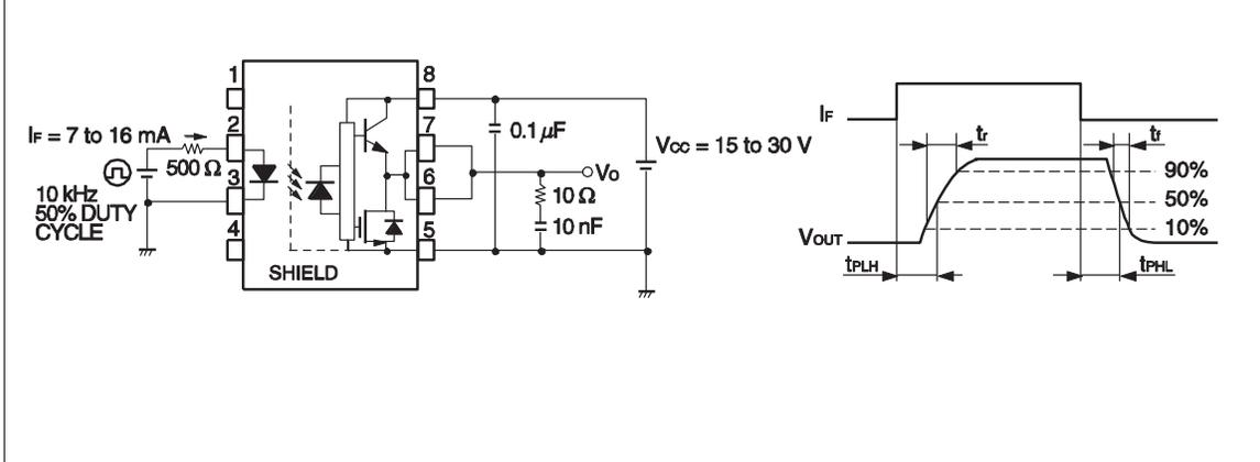
**Fig. 8 CMR Test Circuit and Wave Forms**
