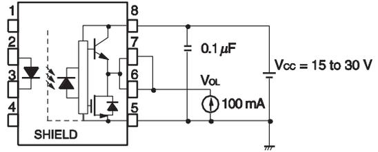
Fig. 5 I<sub>FLH</sub> Test Circuit
