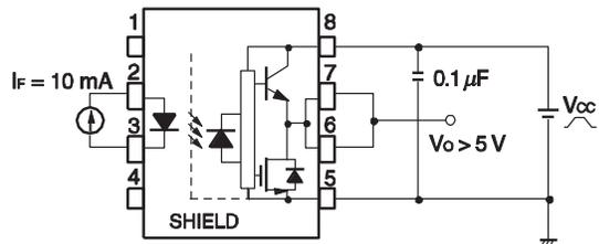
**Fig. 7 t<sub>PLH</sub>, t<sub>PHL</sub>, t<sub>r</sub>, t<sub>f</sub> Test Circuit and Wave Forms**
