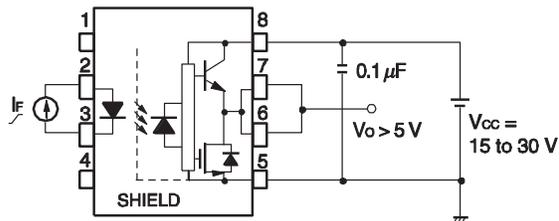
Fig. 6 UVLO Test Circuit
