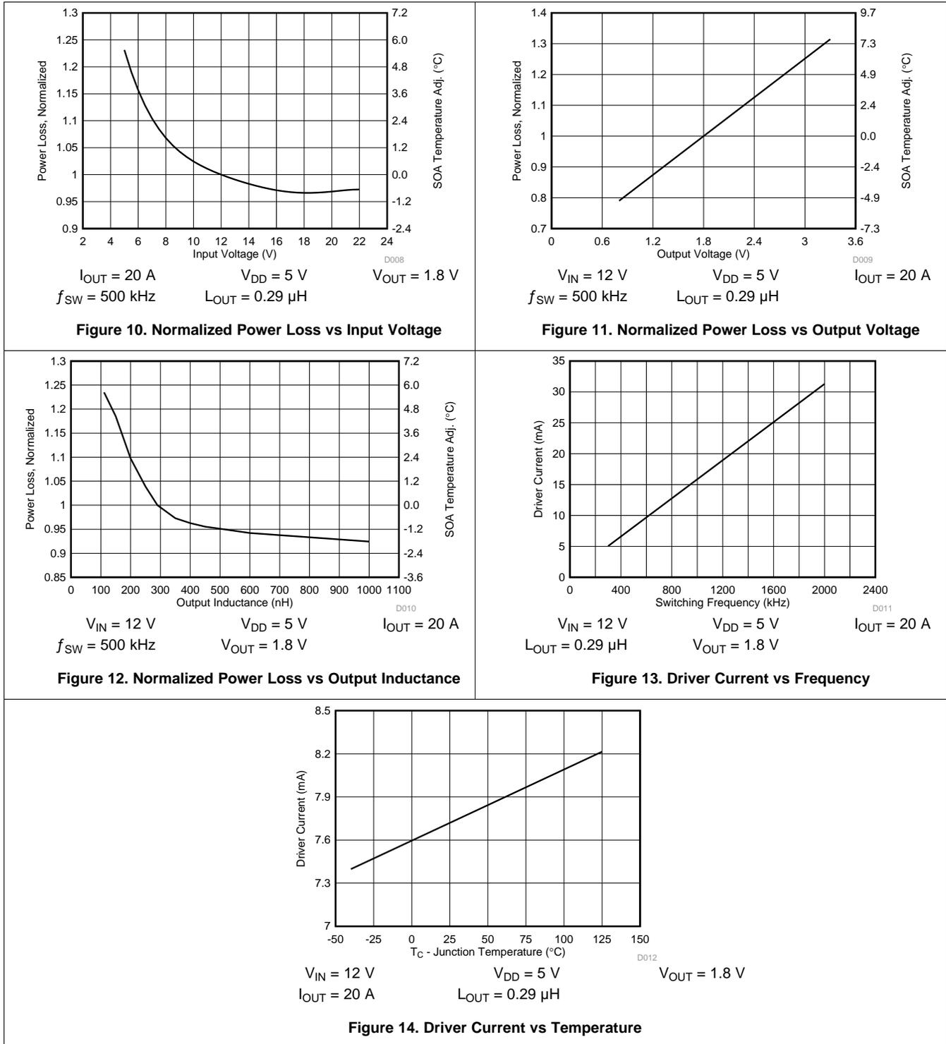
1. The Typical CSD97394Q4M System Characteristic curves are based on measurements made on a PCB design with dimensions of 4.0 inches (W) x 3.5 inches (L) x 0.062 inch (T) and 6 copper layers of 1 oz. copper thickness. See the [System Example](#) section for detailed explanation.
