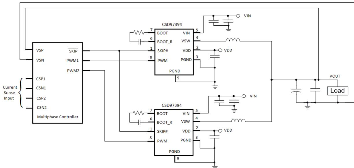
Figure 3. Application Schematic
