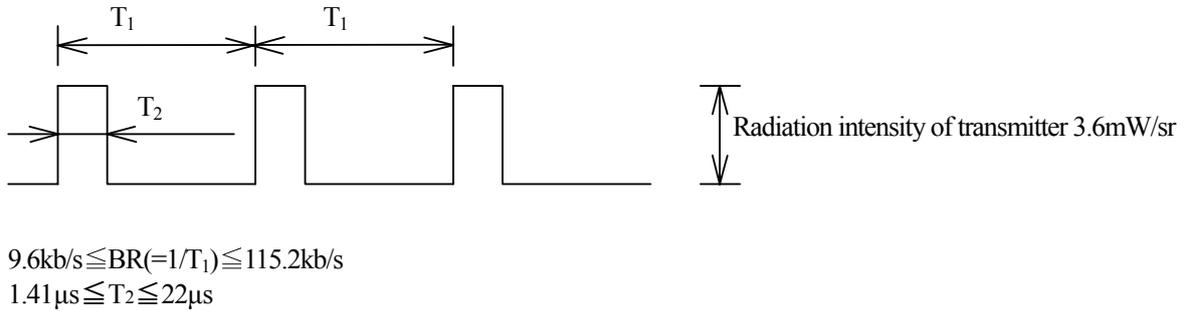
**Fig.3 Output Waveform Specification(Receiver side)**
