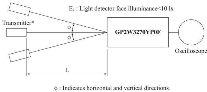
\*Transmitter shall use GP2W3270YP0F ( $\lambda_p=890\text{nm TYP.}$ ) which is adjusted the radiation intensity at  $3.6\text{mW/sr}$ .
