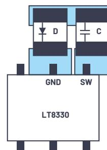
Figure 2. Board layout optimized for the Ćuk topology.
