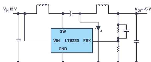
Figure 3. Example of a circuit for a Ćuk regulator with an LT8330.
