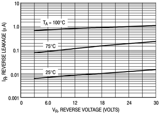
Figure 3. Reverse Leakage
