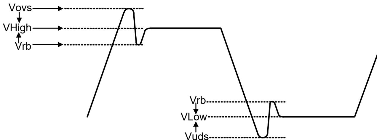
**Figure 5. Single-ended Measurement Points for  $V_{ovs}$ ,  $V_{uds}$ ,  $V_{rb}$**
