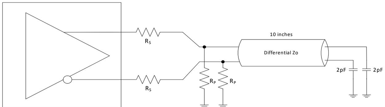
**Figure 7. 0.7 V Configuration Test Load Board Termination**
