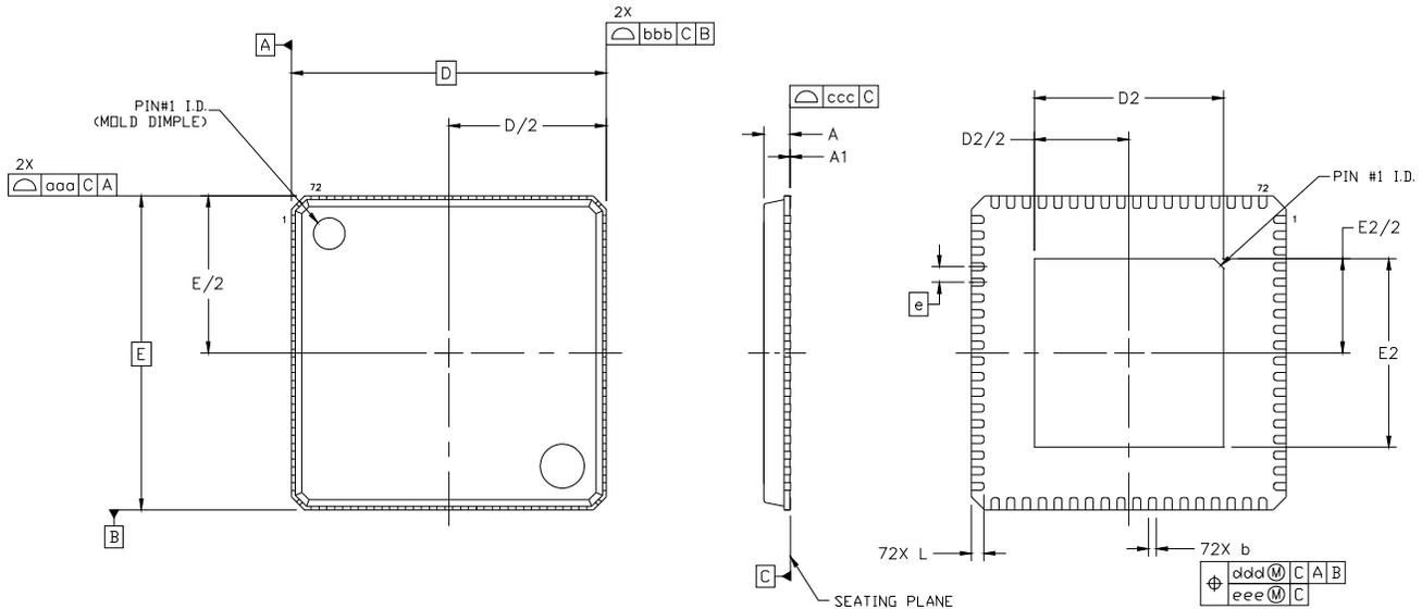
**Figure 13. 72-Pin Quad Flat No Lead (QFN) Package**
