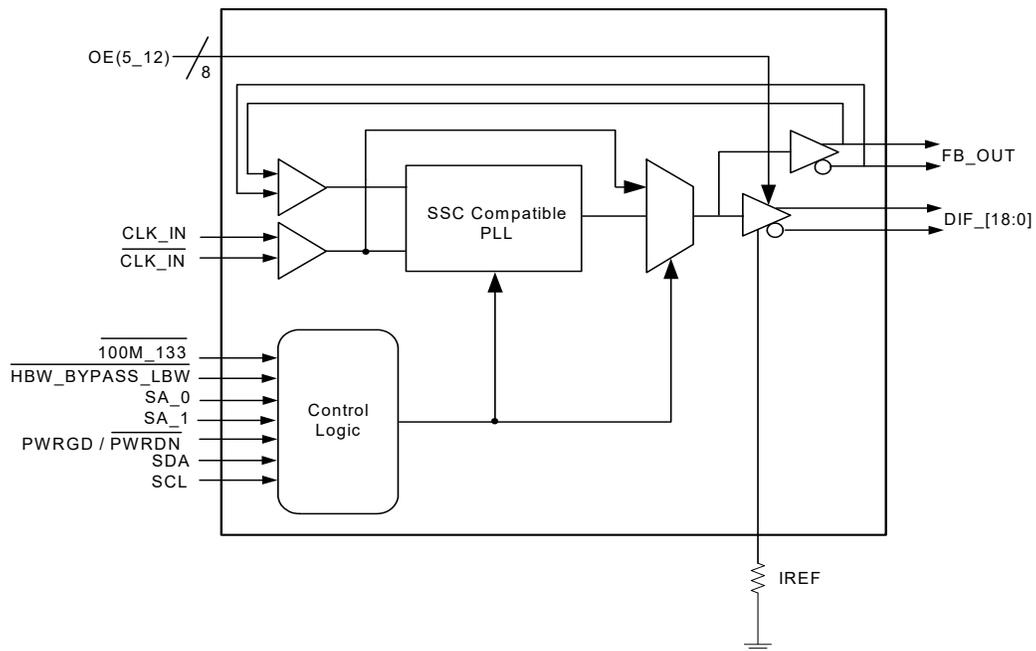
Note: FB\_OUT pins must be identically terminated to the other DIF outputs.
