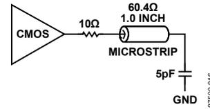
Figure 13. Series Termination of CMOS Output
