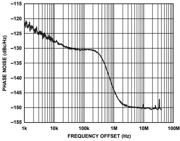
Figure 6. 100 MHz Phase Noise
