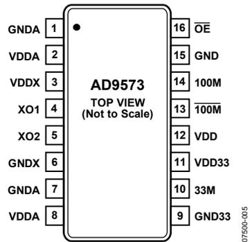
Figure 5. Pin Configuration
