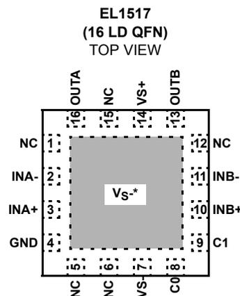
\*THERMAL PAD MUST BE CONNECTED TO NEGATIVE SUPPLY: VS-. QFN PACKAGE CAN BE USED IN DUAL SUPPLY APPLICATIONS.
