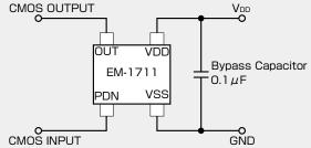
Note1) During power down mode, output is latched in its previous state.
