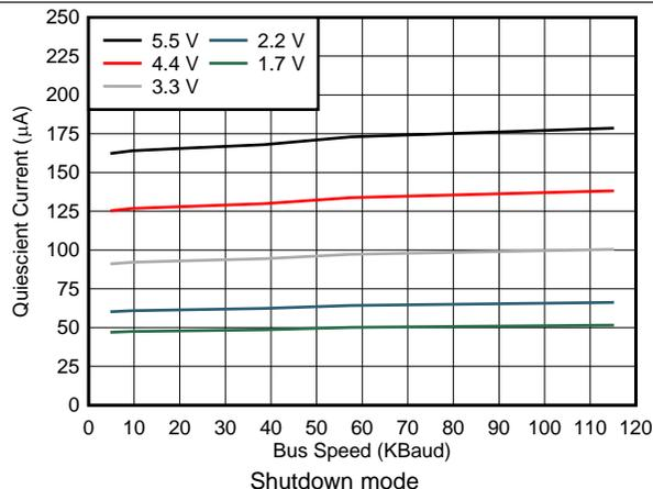
Figure 11. Quiescent Current vs SMA Wire Bus Speed
