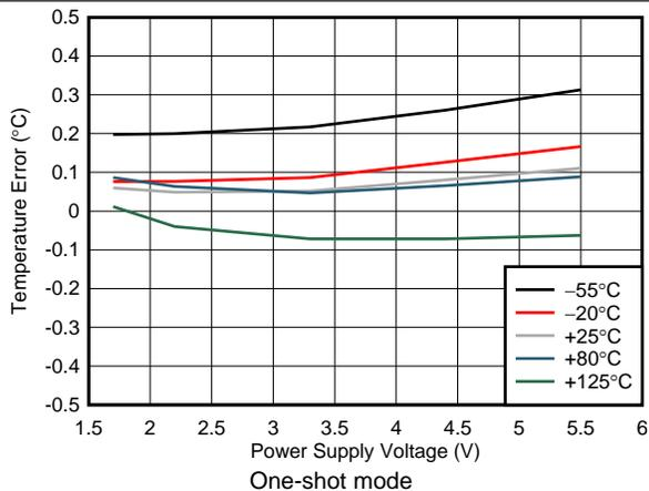
Figure 8. Temperature Error vs Power Supply Voltage
