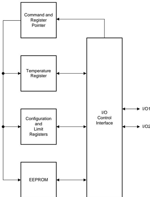
Figure 30. Register Structure
