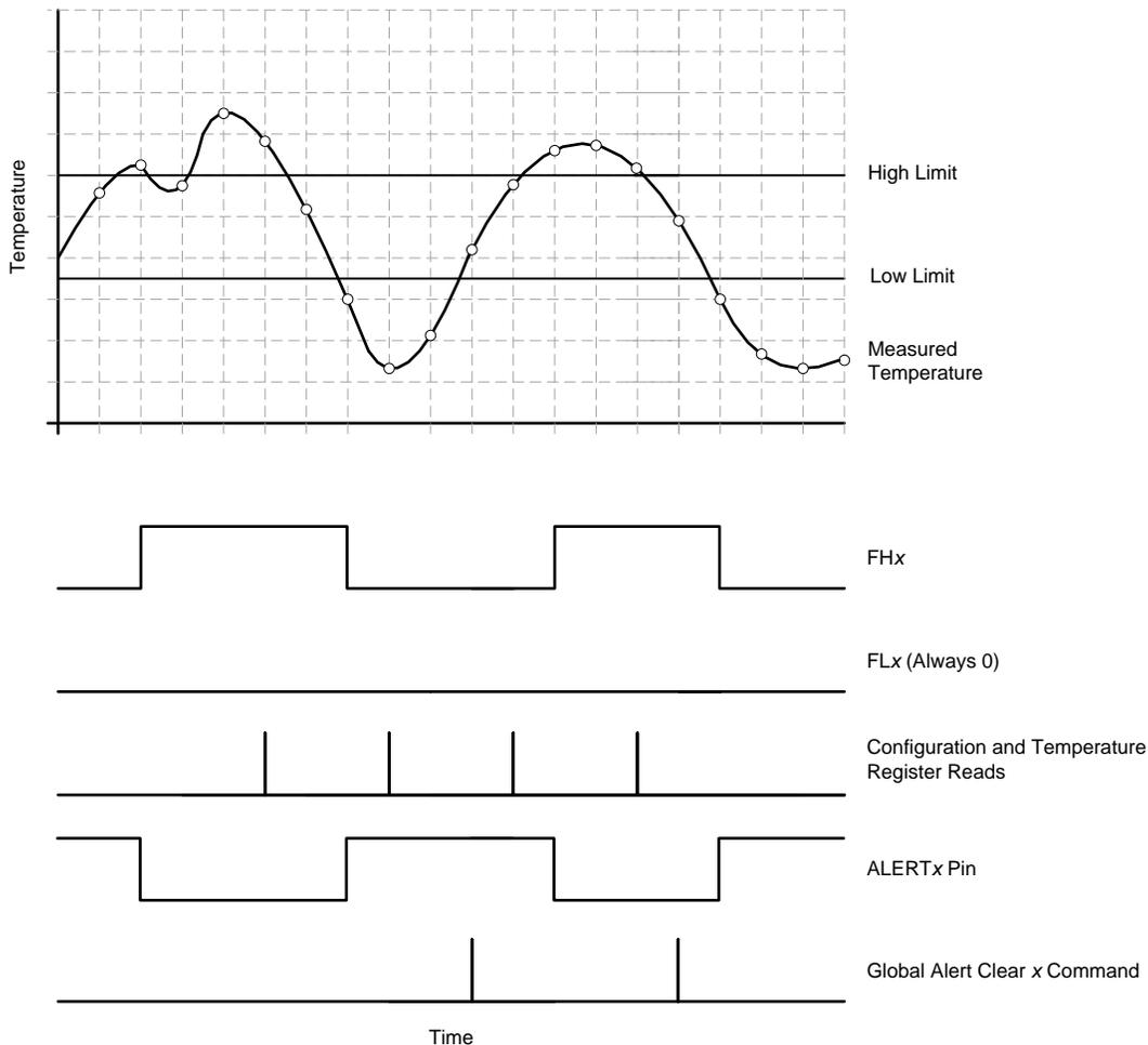
**Figure 17. ALERTx Pin Behavior in Therm Mode (POLx = 0)**
