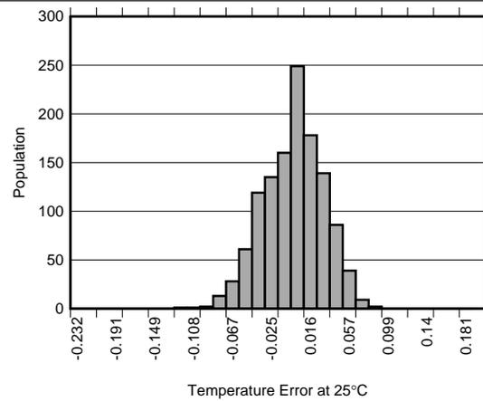
Figure 5. Temperature Error Histogram
