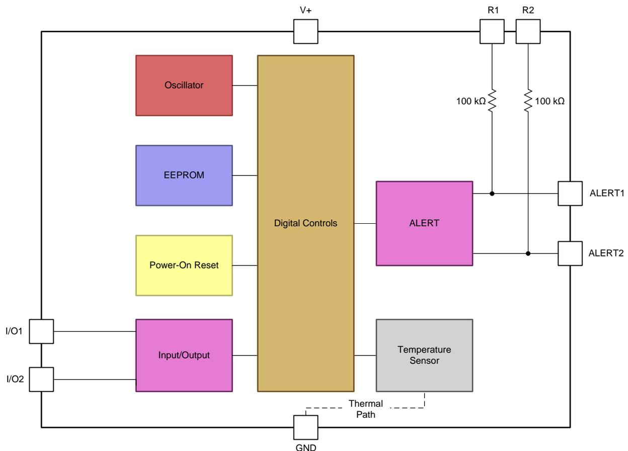
NOTE: The temperature sensor of the TMP107-Q1 is the silicon chip. Thermal paths run through the package leads. The lower thermal resistance of metal enables the leads to provide the primary thermal path.
