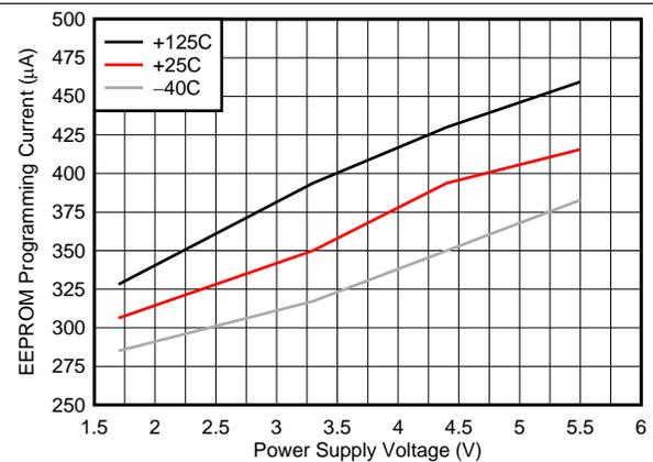
Figure 13. EEPROM Programming (Write) Current vs Power Supply Voltage
