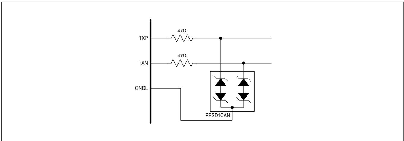
Figure 25. Supplemental ESD Protection for UART Transmitter
