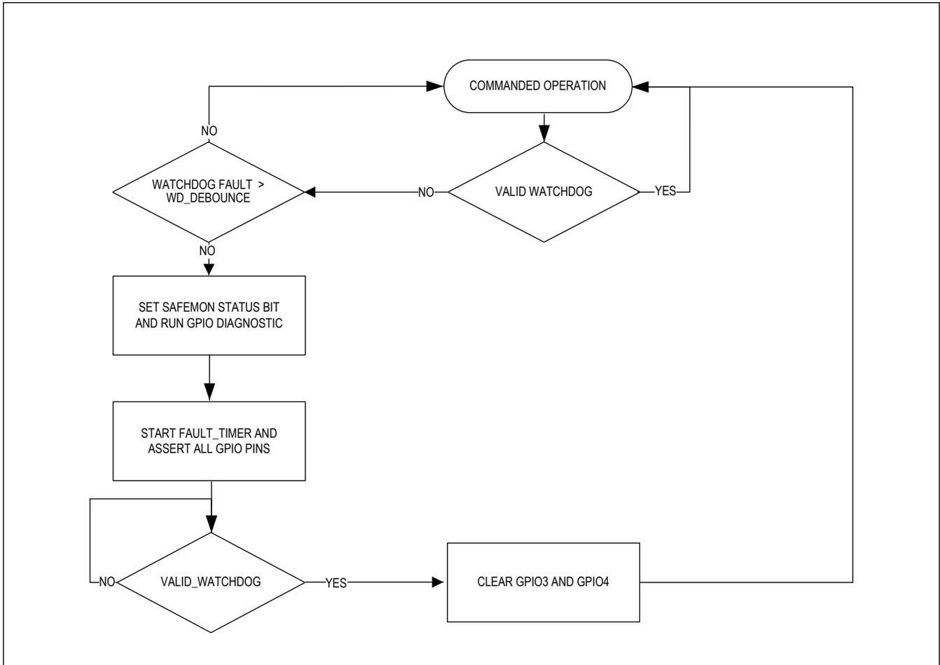
Figure 8. BMS Safe Monitoring (NOMON) Mode Flow Chart
