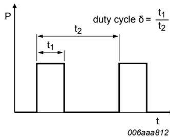
Fig. 17. Duty cycle definition
