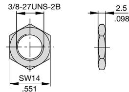
This is a metric design and millimeter dimensions take precedence ( $\frac{mm}{inch}$ )
