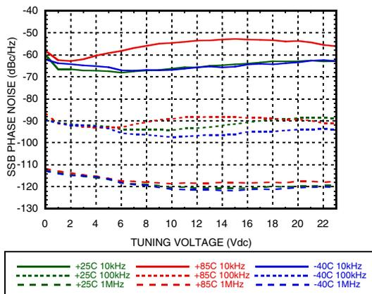
**Typical SSB Phase Noise @ Vtune = +10V**
