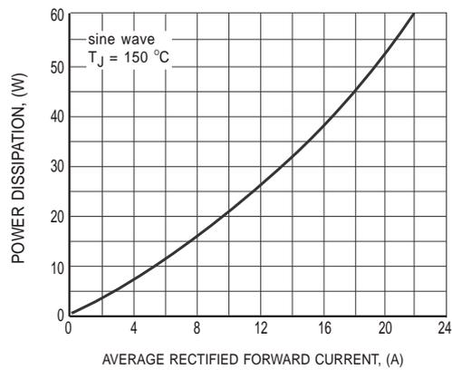
FIG.2 POWER DISSIPATION
