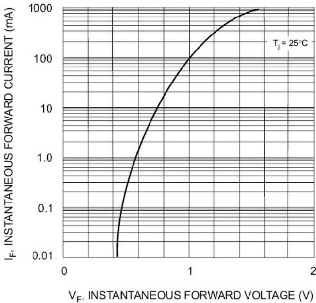
Fig. 1 Forward Characteristics
