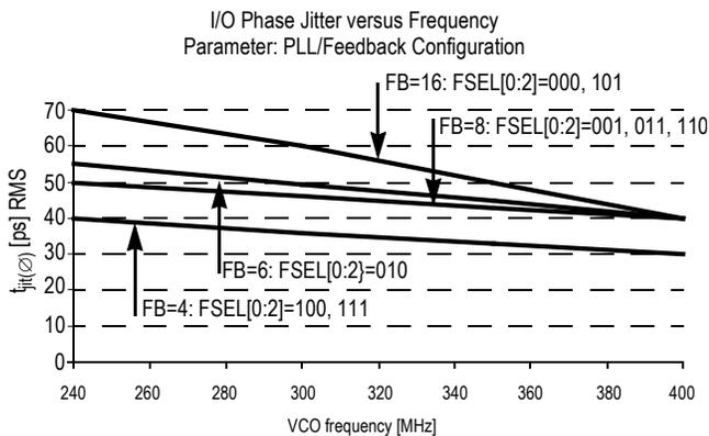
**Figure 5. Max. I/O Phase Jitter versus VCO Frequency**
