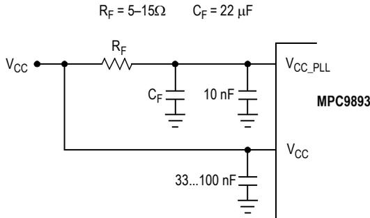
**Figure 3. V<sub>CC\_PLL</sub> Power Supply Filter**
