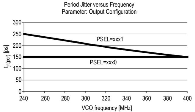
**Figure 7. Max. Period Jitter versus VCO Frequency**
