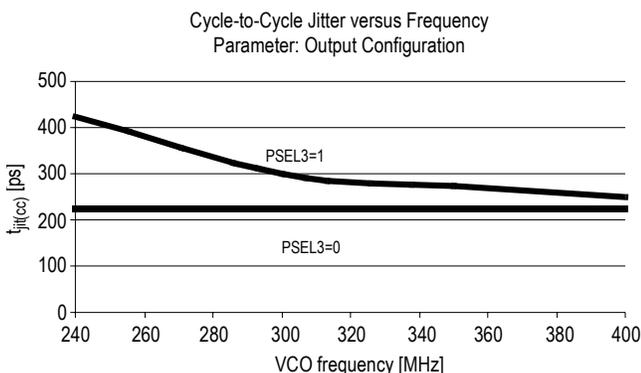
**Figure 6. Max. Cycle-to-Cycle Jitter versus VCO Frequency**
