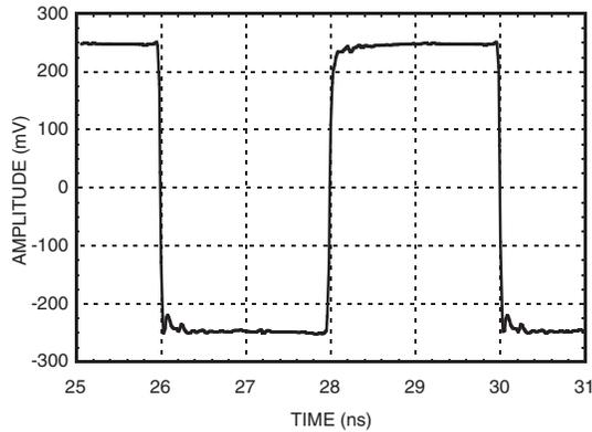
**Output Voltage Waveform,  $F_{in} = 750$  MHz,
