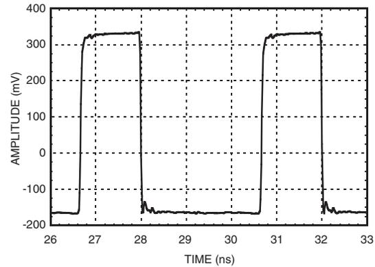
**Output Voltage Waveform,  $F_{in} = 2500$  MHz,
