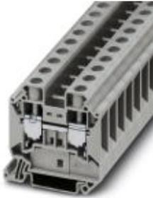
Feed-through terminal block, Connection method: Screw connection, Cross section: 1.5 mm<sup>2</sup> - 25 mm<sup>2</sup>, AWG: 16 - 4, Width: 12.2 mm, Height: 54.4 mm, Color: black, Mounting type: NS 35/7,5, NS 35/15
