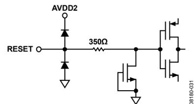
Figure 37. Equivalent RESET Input Circuit
