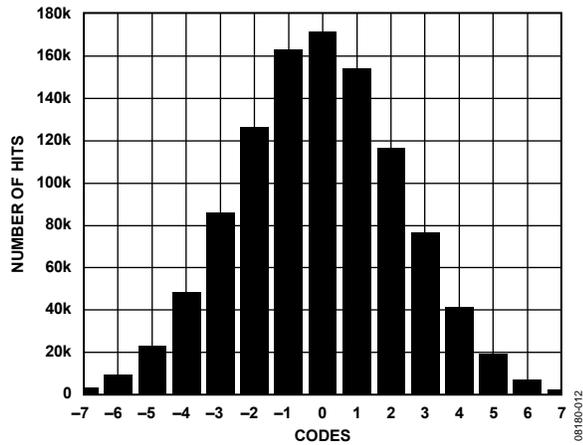
Figure 12. Output-Referred Noise Histogram, GAIN+ = 1.6 V
