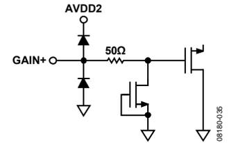
Figure 41. Equivalent GAIN+ Input Circuit
