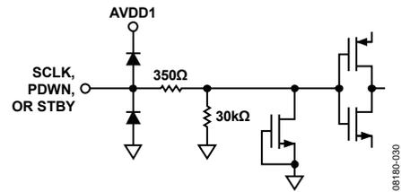
Figure 36. Equivalent SCLK, PDWN, or STBY Input Circuit
