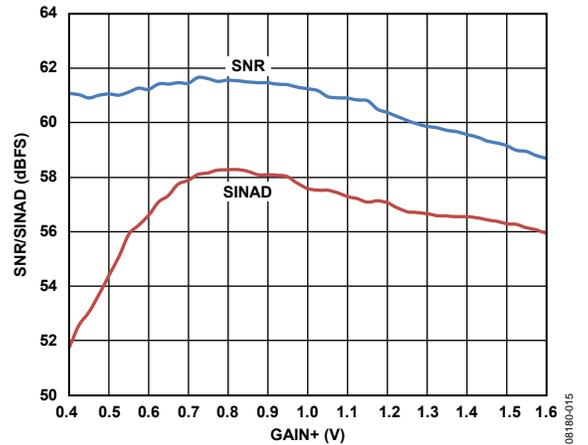
Figure 15. SNR/SINAD vs. GAIN+, AIN = -1.0 dBFS
