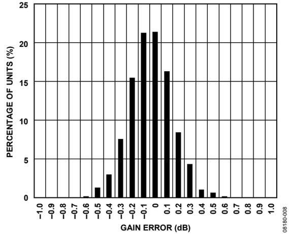
Figure 8. Gain Error Histogram, GAIN+ = 1.44 V
