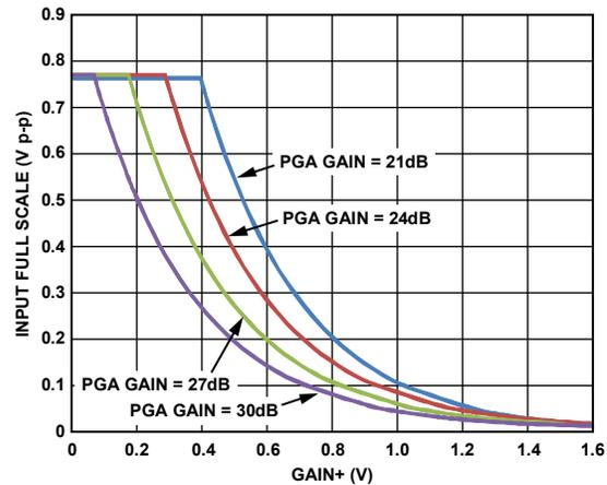
Figure 56. LNA with 15.6 dB Gain Setting/VGA Full-Scale Limitations
