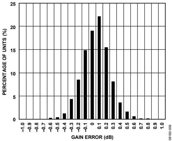
Figure 6. Gain Error Histogram, GAIN+ = 0.16 V
