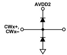
Figure 43. Equivalent CWI±, CWQ± Output Circuit
