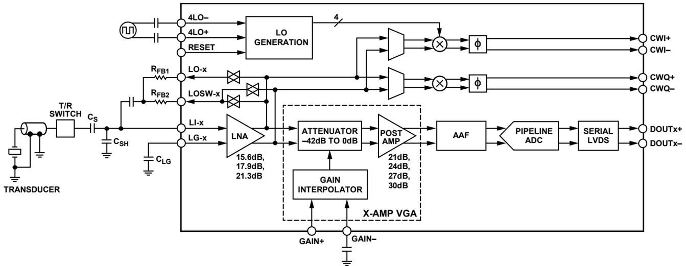
Figure 46. Simplified Block Diagram of a Single Channel
