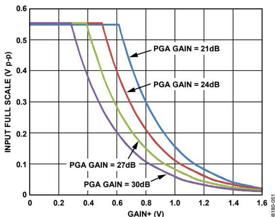
Figure 57. LNA with 17.9 dB Gain Setting/VGA Full-Scale Limitations
