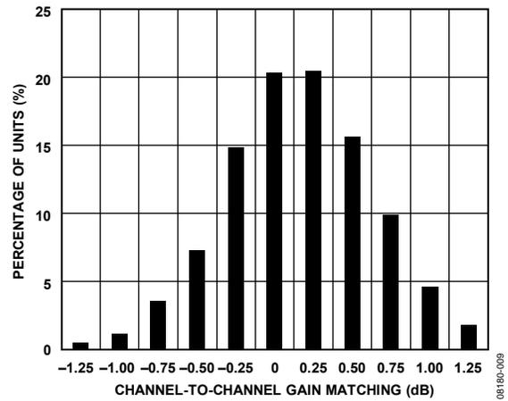
Figure 9. Gain Match Histogram, GAIN+ = 0.3 V
