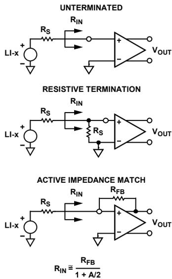
Figure 49. Input Configurations
