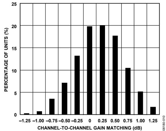
Figure 10. Gain Match Histogram, GAIN+ = 1.3 V
