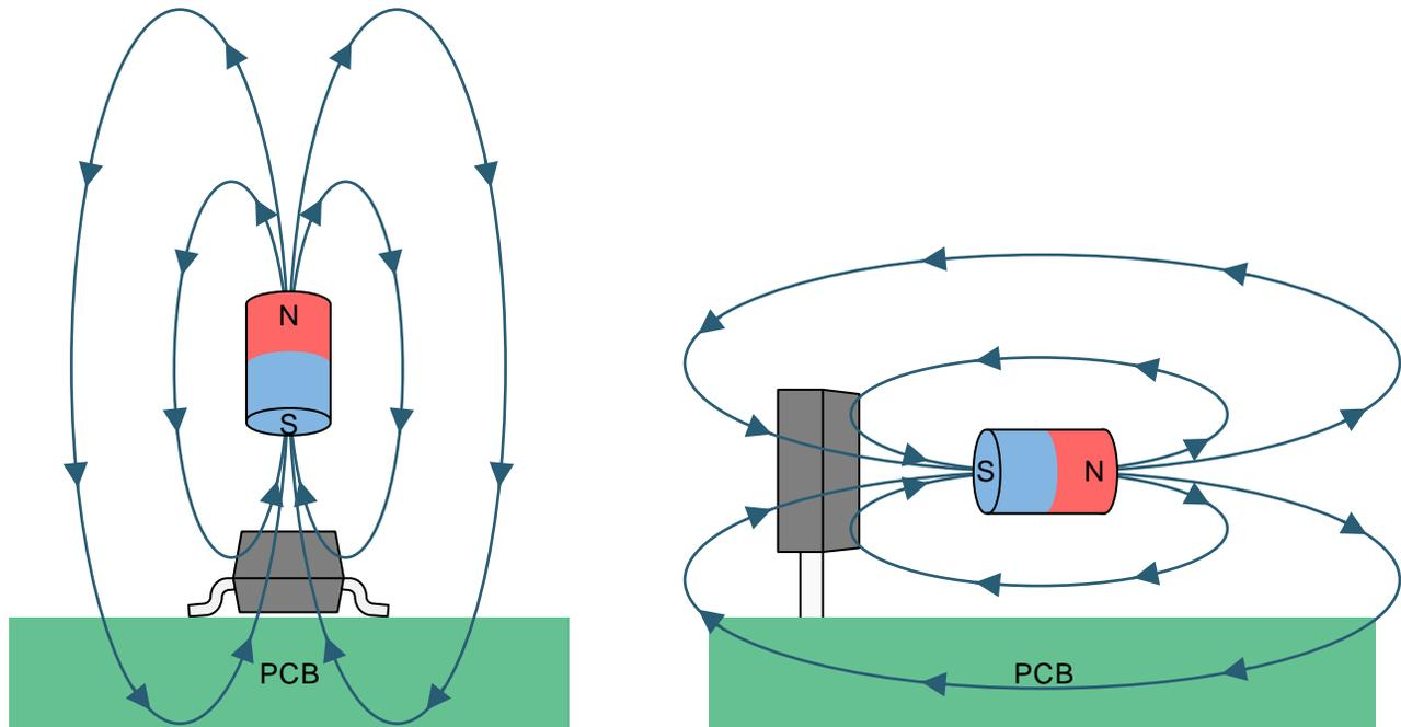
**Figure 15. The Flux Direction for Positive B**
