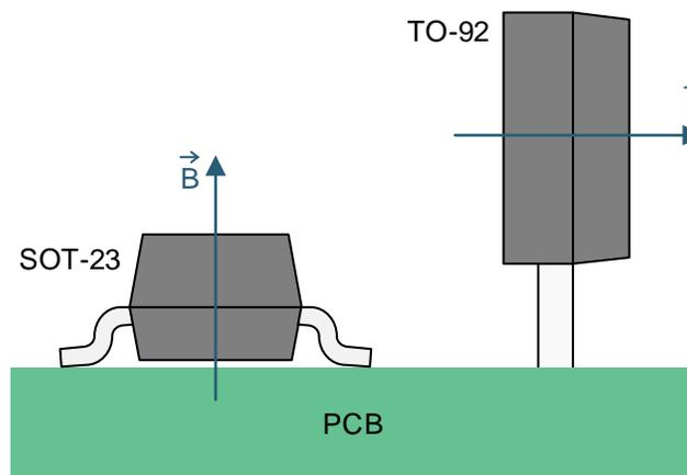
Figure 14. Direction of Sensitivity
