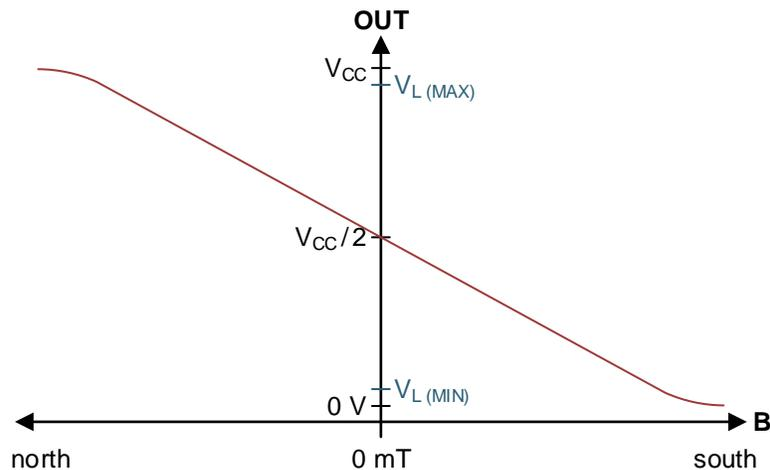
Figure 17. Magnetic Response of the A5 Version
