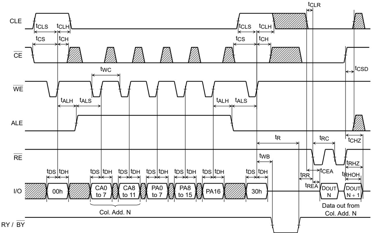
Read Cycle with Data Cache Timing Diagram (1/2)
