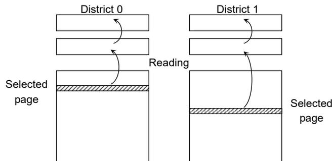
The data transfer operation from the cell array to the Data Cache via Page Buffer starts on the rising edge of  $\overline{WE}$  in the 30h command input cycle (after the 2 Districts' address information has been latched).
