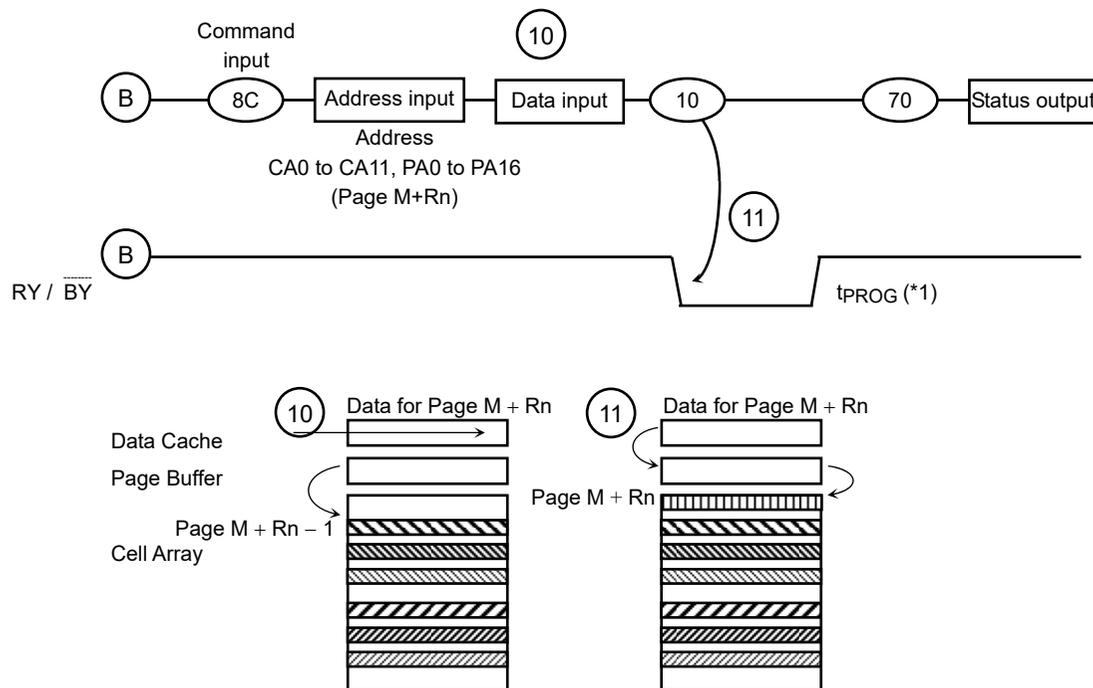
10. Address for Page (M + Rn) is input. If the data needs to be changed, changed data is input.
