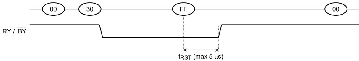
When a Reset (FFh) command is input during Ready
