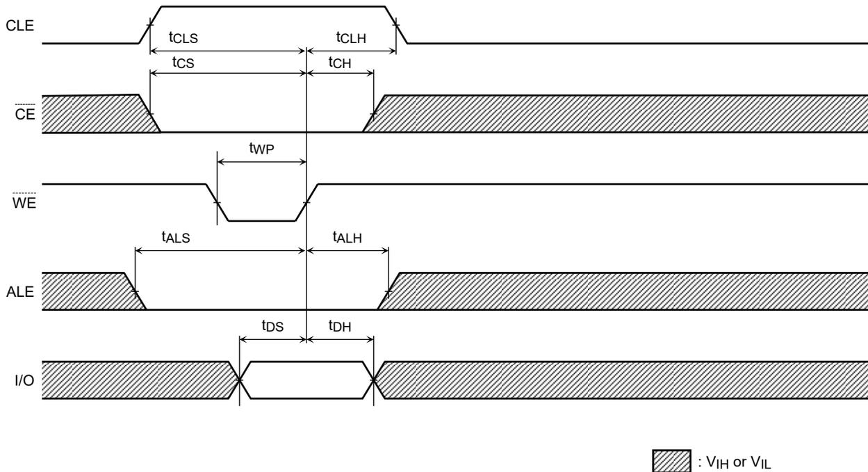
Address Input Cycle Timing Diagram
