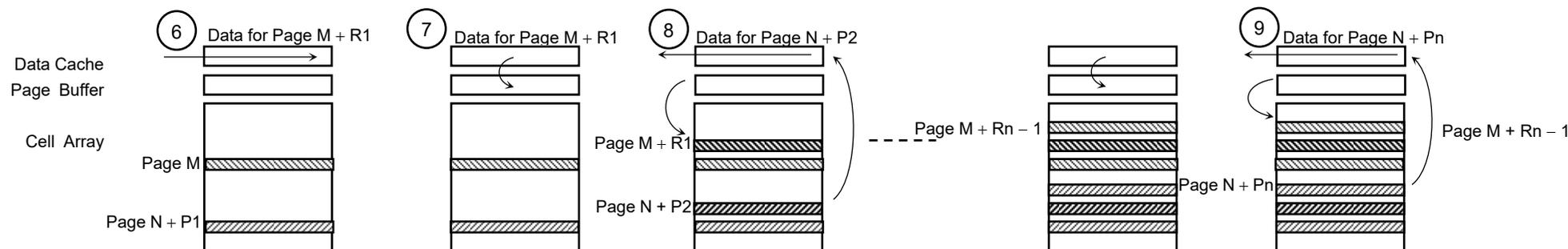
6. Address for Page (M + R1) is input. If the data needs to be changed, changed data is input.
