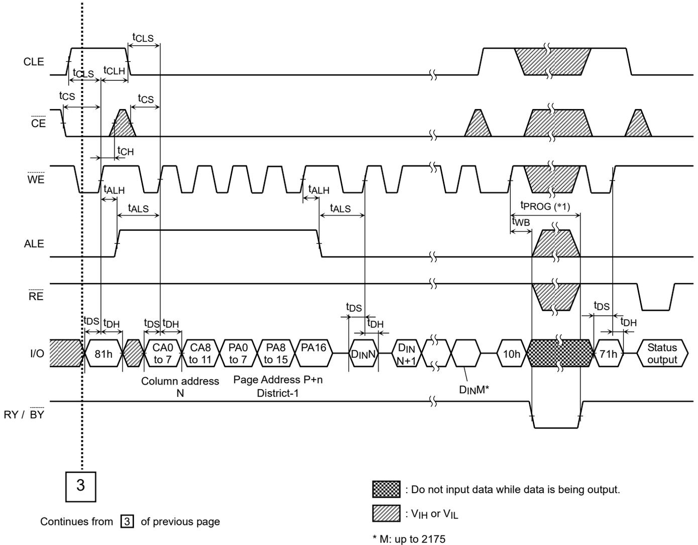
(\*1) t<sub>PROG</sub>: Since the last page's programming by 10h command is initiated after the previous cache program, the t<sub>PROG</sub> during cache programming is given by the following equation.
