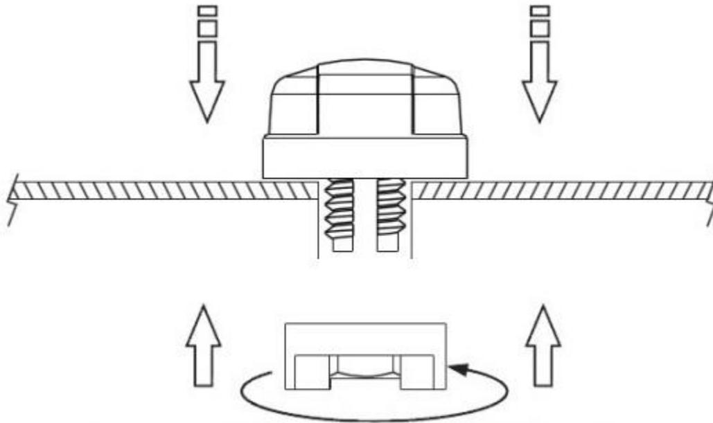
Recommended torque for Mounting is 24.5N·m
