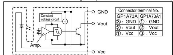
\* GP1A73A and GP1A73A1 are different in the terminal marking number of connectors from each other due to use of connectors of different manufacturers.
