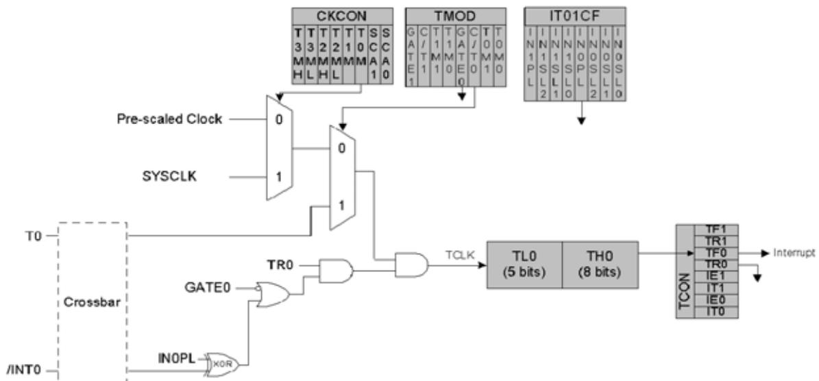
**Figure 24.1. T0 Mode 0 Block Diagram**
