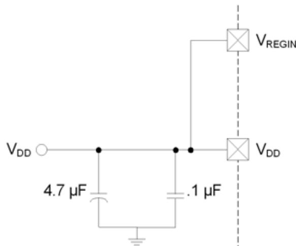
**Figure 8.2. External Capacitors for Voltage Regulator Input/Output**
