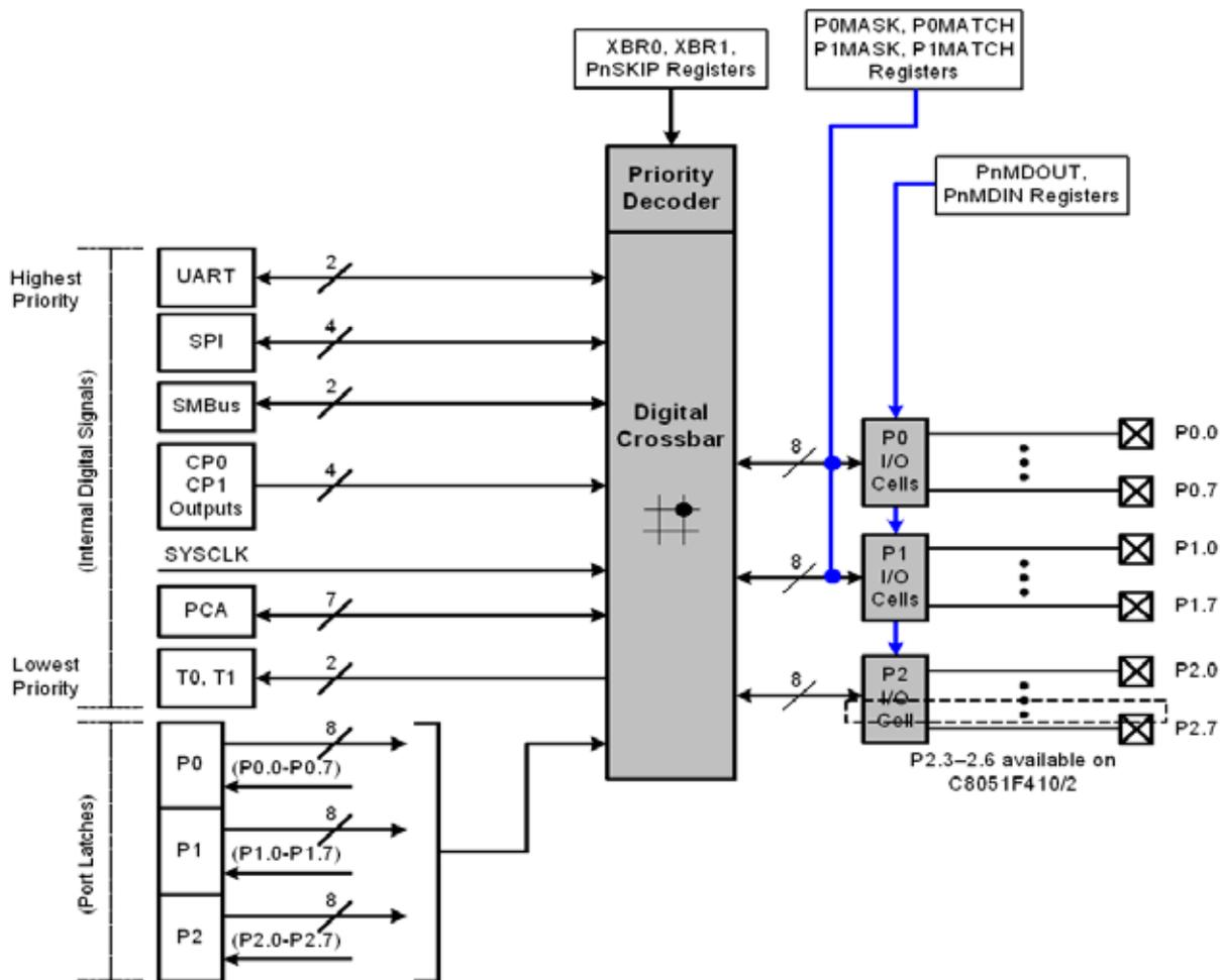
Figure 18.1. Port I/O Functional Block Diagram
