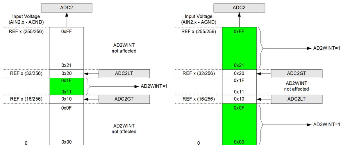
Figure 7.5. ADC2 Window Compare Examples, Single-Ended Mode
