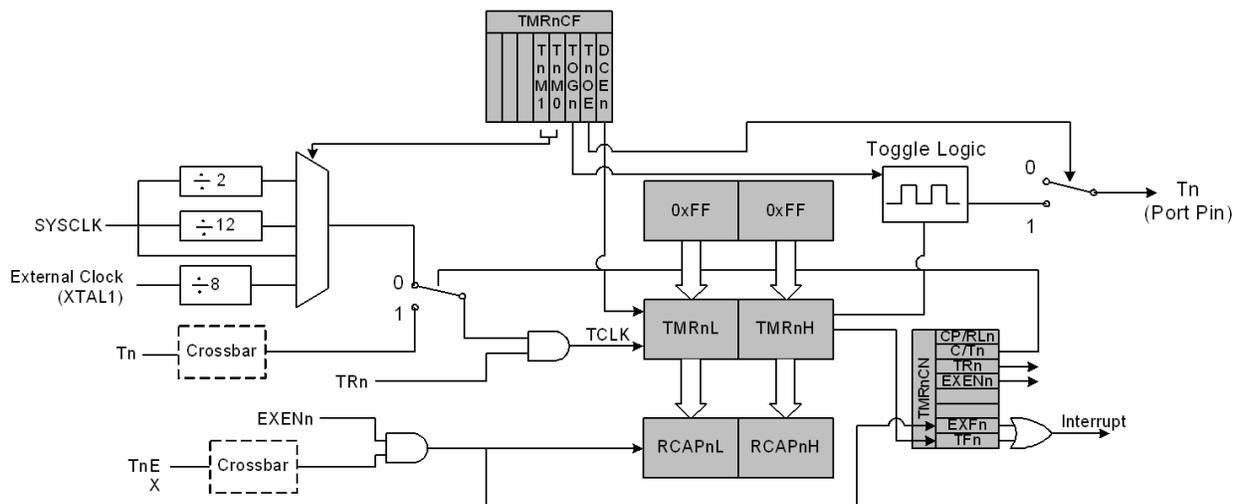
**Figure 23.4. T2, 3, and 4 Capture Mode Block Diagram**
