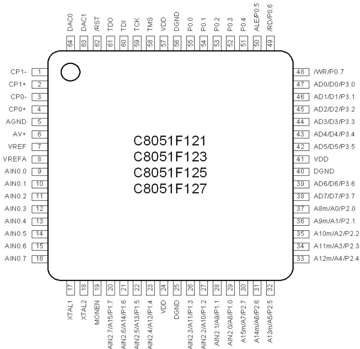
Figure 4.4. C8051F121/3/5/7 Pinout Diagram (TQFP-64)
