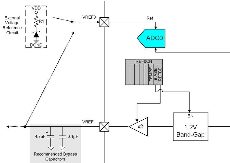
**Figure 9.3. Voltage Reference Functional Block Diagram (C8051F130/1/2/3)**
