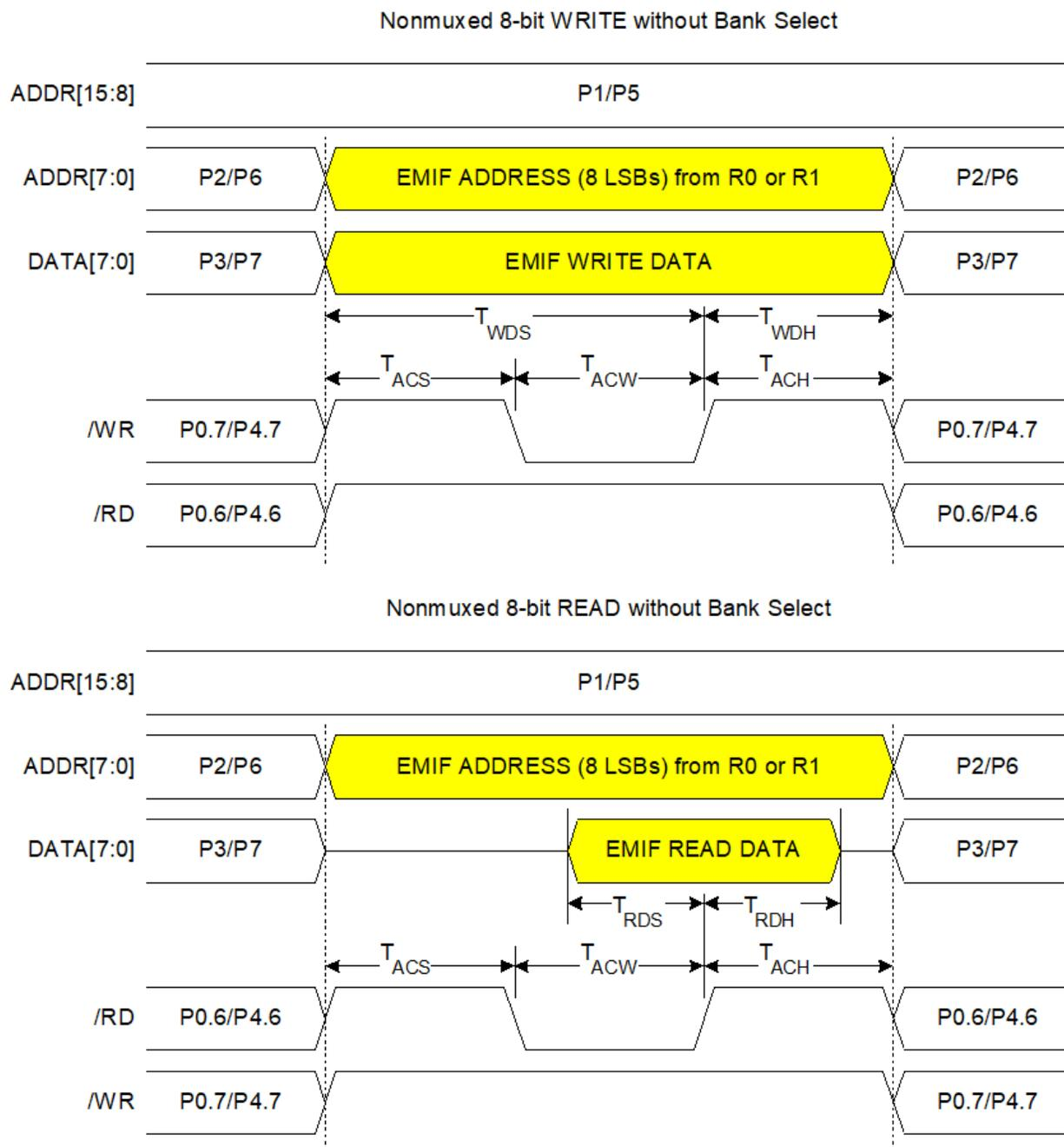
**Figure 17.5. Non-multiplexed 8-bit MOVX without Bank Select Timing**
