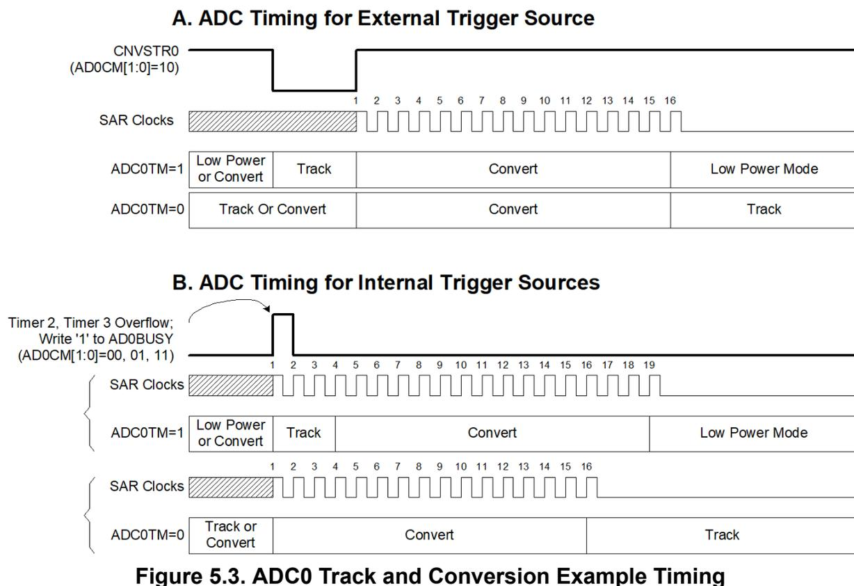
**Figure 5.3. ADC0 Track and Conversion Example Timing**
