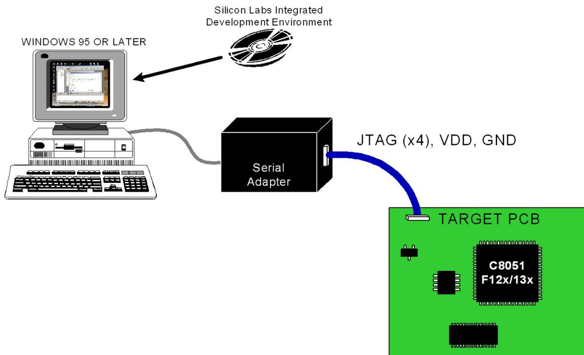
Figure 1.9. Development/In-System Debug Diagram
