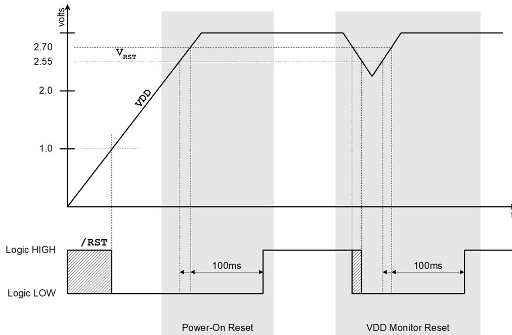
Figure 13.2. Reset Timing
