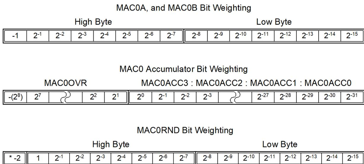
\* The MAC0RND register contains the 16 LSBs of a two's complement number. The MAC0N Flag can be used to determine the sign of the MAC0RND register.
