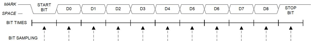
Figure 21.5. UART0 Modes 2 and 3 Timing Diagram
