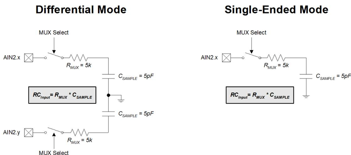
Note: When the PGA gain is set to 0.5, C<sub>SAMPLE</sub> = 3pF
