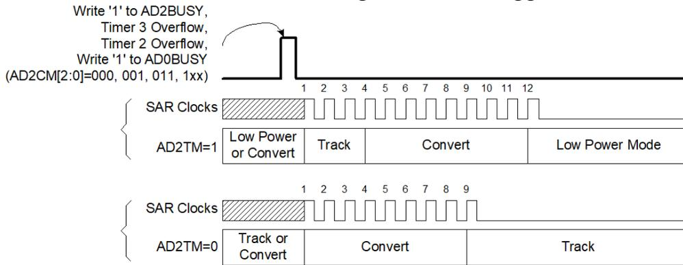
**Figure 7.2. ADC2 Track and Conversion Example Timing**
