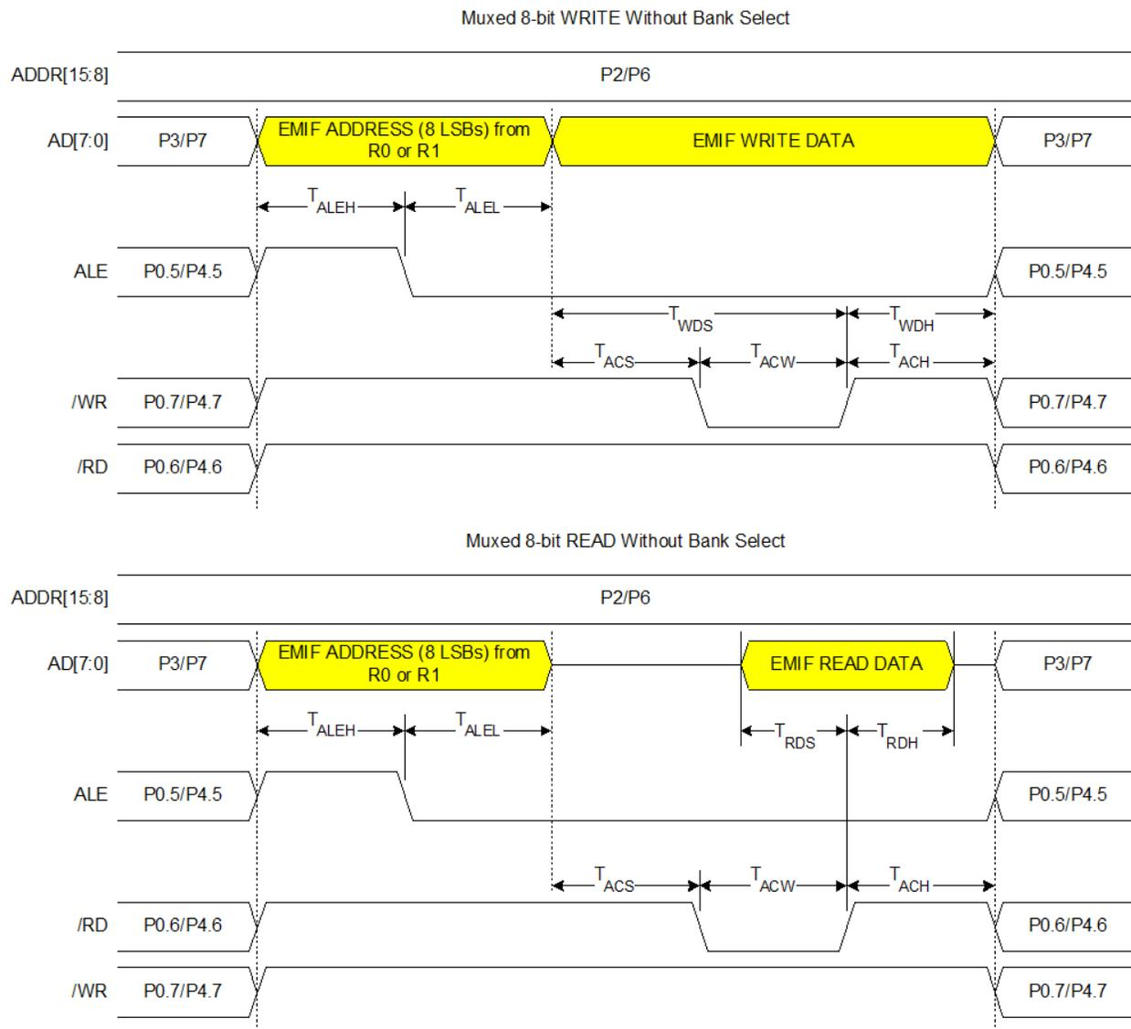
**Figure 17.8. Multiplexed 8-bit MOVX without Bank Select Timing**
