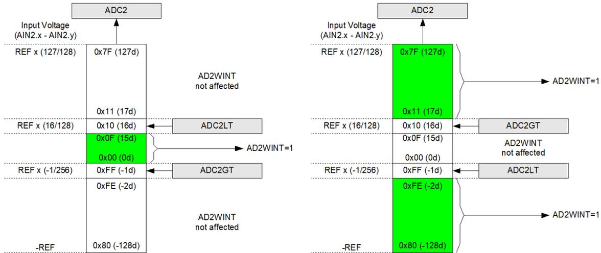
Figure 7.6. ADC2 Window Compare Examples, Differential Mode
