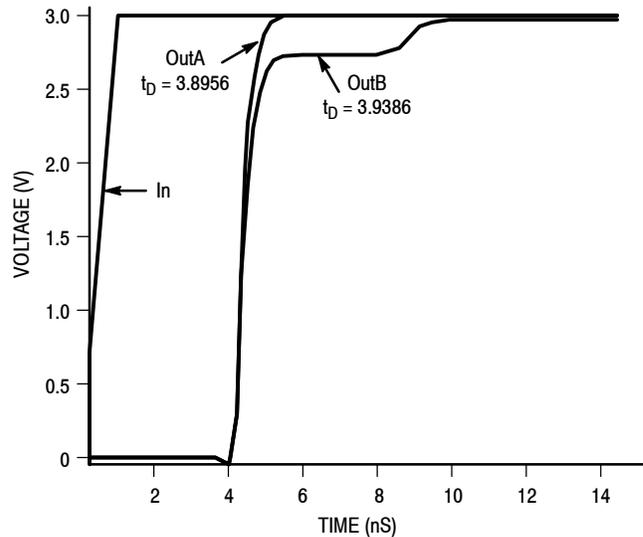
Figure 5. Single versus Dual Line Termination Waveforms
