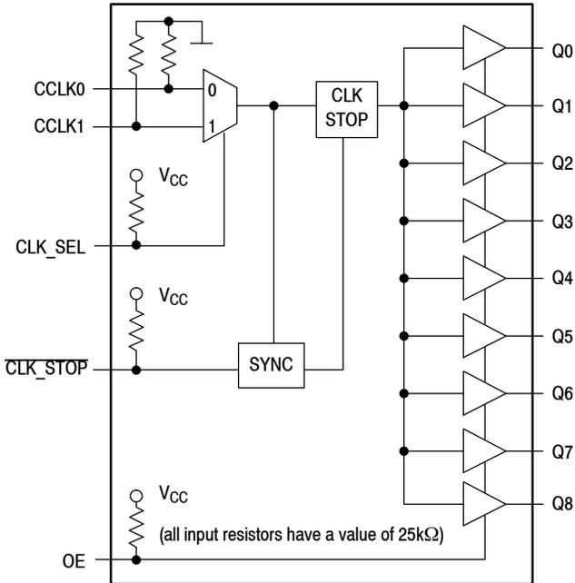
Figure 1. Logic Diagram
