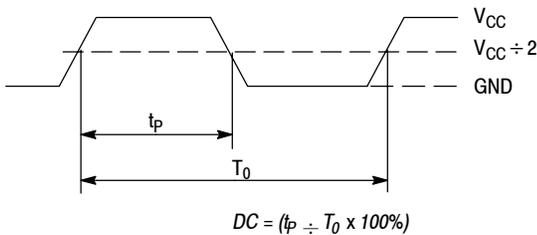
The time from the output controlled edge to the non-controlled edge, divided by the time between output controlled edges, expressed as a percentage
