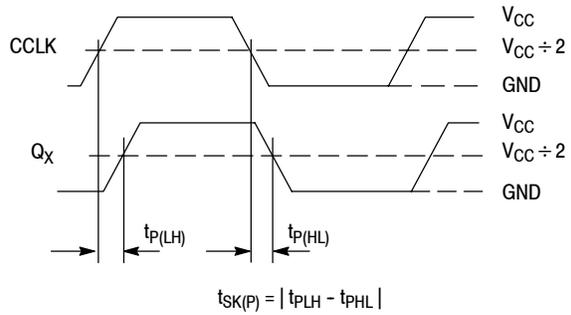
Figure 10. Output Pulse Skew ( $t_{SK(P)}$ ) Test Reference
