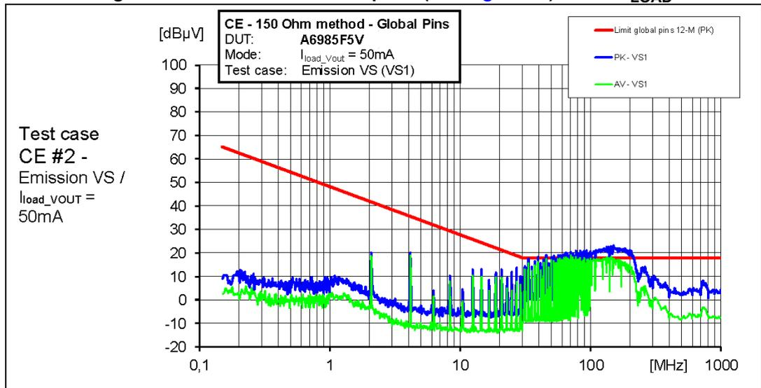
Figure 69. CE 150R at VOUT test point (see Figure 66) at 75% I<sub>LOAD</sub>
