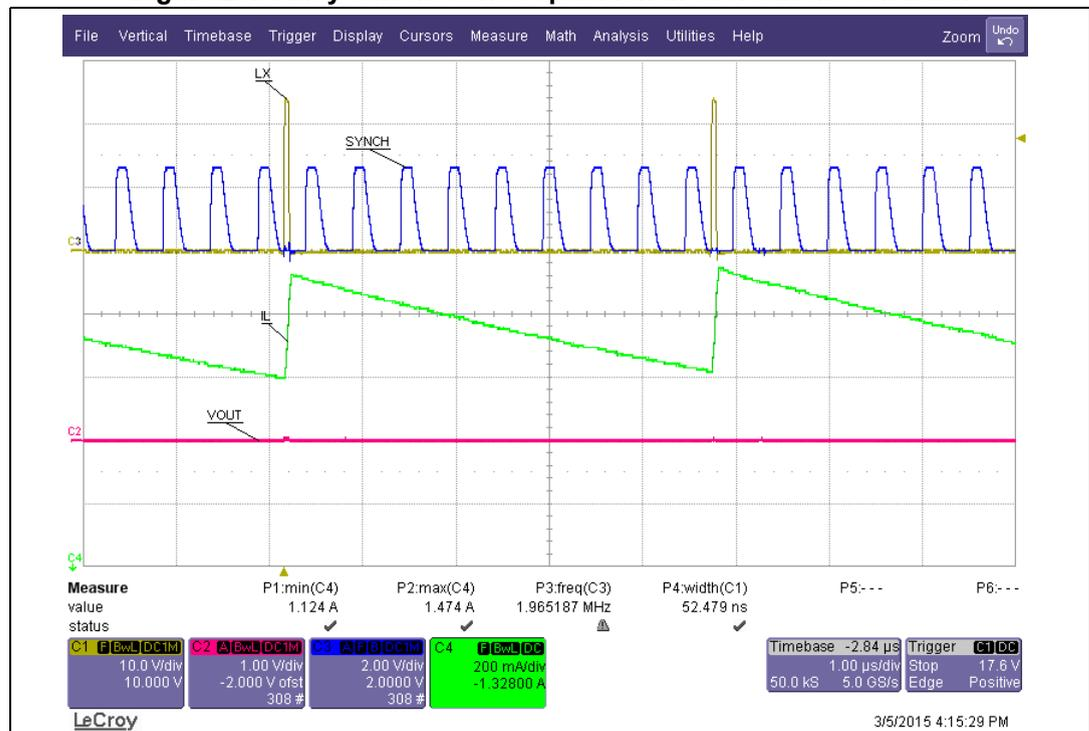
Figure 29 shows the switching frequency reduction during the valley current sense operation in case of extremely low duty cycle ( $V_{IN} = 38\text{ V}$ ,  $f_{SW} = 2\text{ MHz}$  short-circuit condition).
