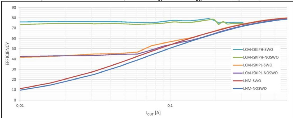
Figure 64. A6985F5V efficiency curves:  $V_{IN} = 24\text{ V}$  -  $f_{sw} = 2\text{ MHz}$
