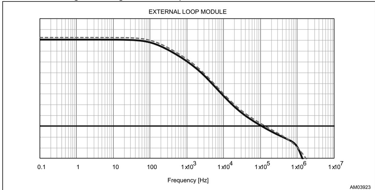
Figure 55. Phase margin Bode's plot of A6985F5V evaluation board
