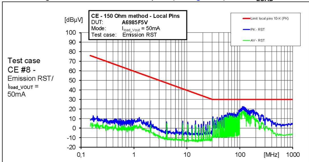
Figure 73. CE 150R at SS/INH test point (see [Figure 66 on page 74](#)) at 75% I<sub>LOAD</sub>
