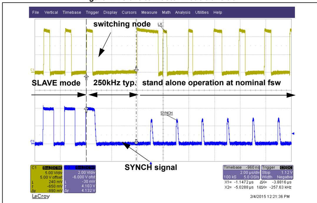
The external master can force a latched SLAVE mode driving the SYNCH pin low at power-up, before the soft-start starts the switching activity. So the oscillator frequency is 250 kHz typ. fixed until a new UVLO event is triggered regardless FSW resistor value, that otherwise counts to design the slope compensation. The same considerations above are also valid.
