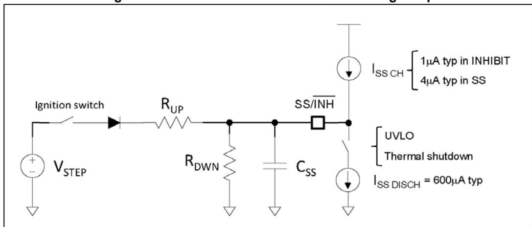
The maximum capacitor value has to be limited to guarantee the device can discharge it in case of thermal shutdown and UVLO events (see [Section 5.3.1](#)), so restart the switching activity ramping the error amplifier reference voltage.
