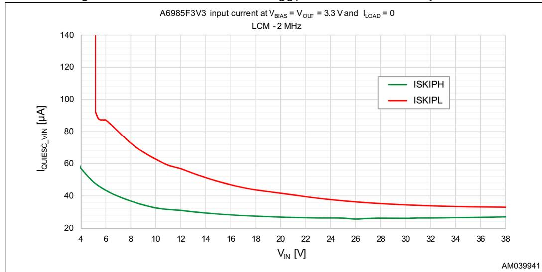
When  $V_{IN}$  is adequately higher than  $V_{OUT}$  (see [Figure 25](#) and [Figure 26](#)), the device works in the bursts mode operation, minimizing the power consumption (see [Section 5.8.2: Low consumption mode \(LCM\)](#)).
