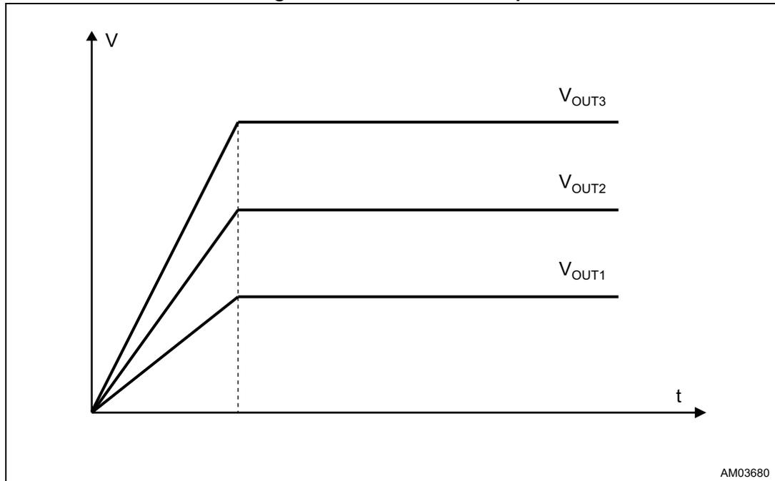
As a consequence all the internal current generators charge in parallel the external capacitor. The capacitor value is dimensioned accordingly with [Equation 12](#):
