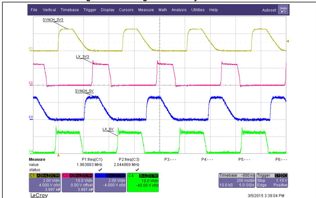
Figure 44 shows the same regulators working synchronized. The MASTER regulator (LX\_5V trace) delivers the synchronization signal (SYNCH\_3V3, SYNCH\_5V pins are connected together) to the SLAVE device (LX\_3V3). The SLAVE regulator works in phase with the synchronization signal which is out of phase with the MASTER switching operation.
