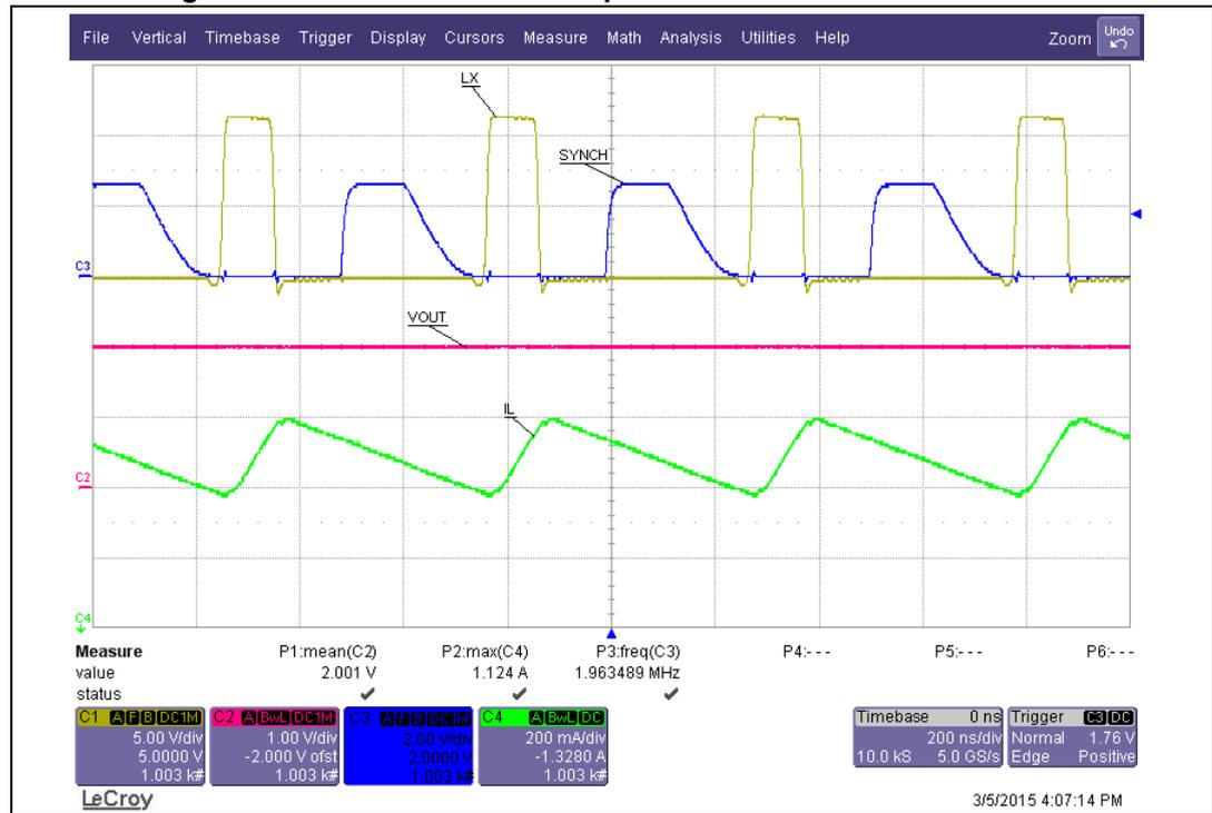
The DC current flowing in the load in overcurrent condition is:
