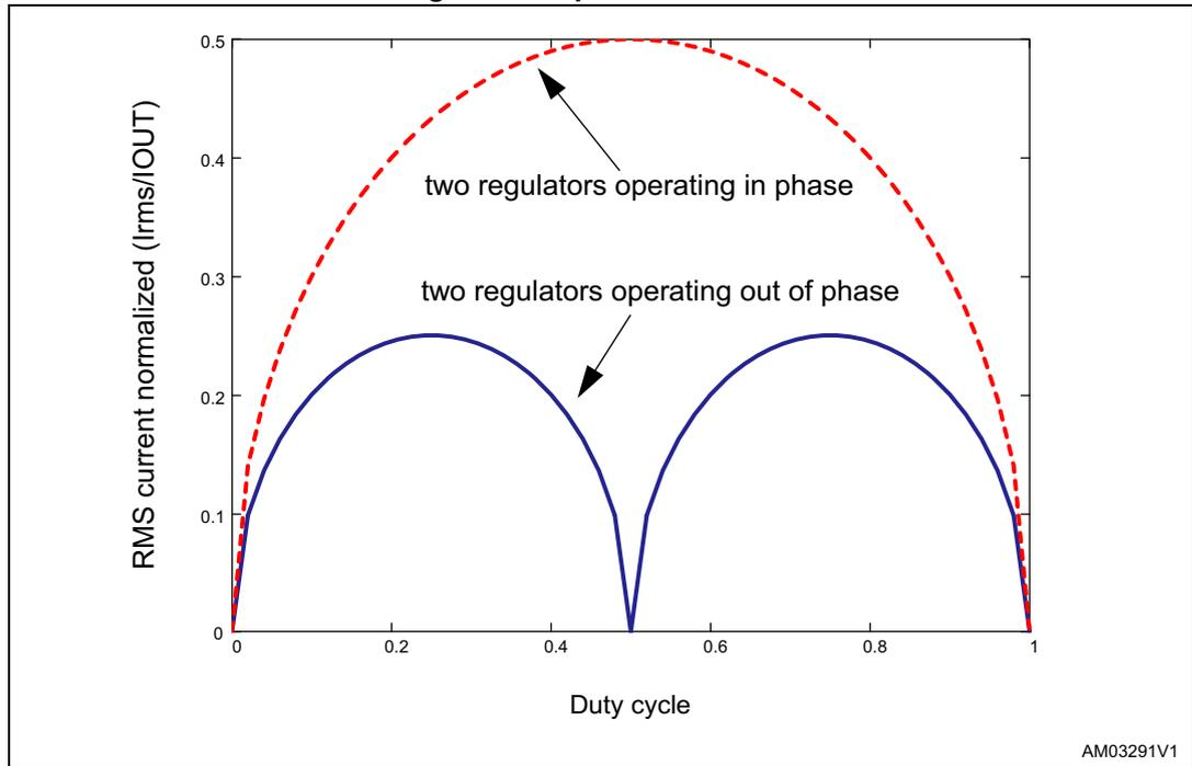
Figure 43 shows two regulators not synchronized.
