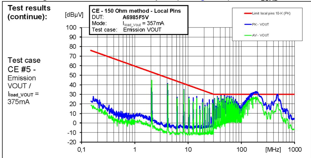
Figure 70. CE 150R at VOUT test point (see Figure 66) at 10% I<sub>LOAD</sub>
