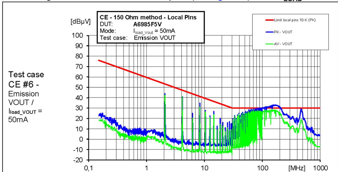
Figure 71. CE 150R at RST test point (see Figure 66) at 75% I<sub>LOAD</sub>
