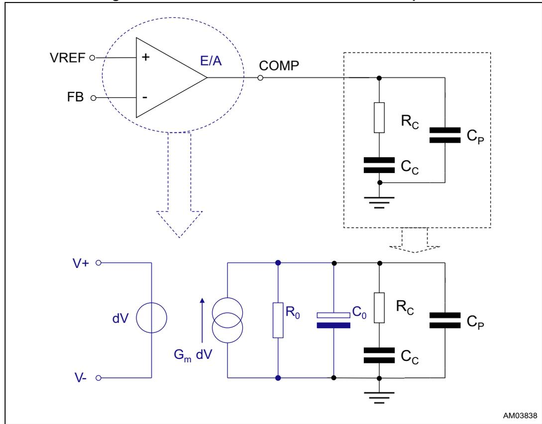
$R_C$  and  $C_C$  introduce a pole and a zero in the open loop gain.  $C_P$  does not significantly affect system stability but it is useful to reduce the noise at the output of the error amplifier.
