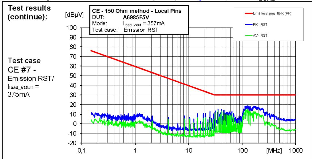
Figure 72. CE 150R at RST test point (see Figure 66) at 10% I<sub>LOAD</sub>
