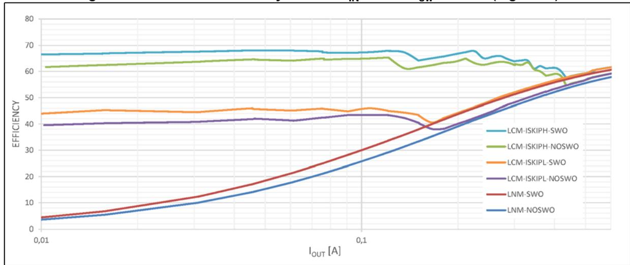
Figure 62. A6985F5V efficiency curves:  $V_{IN} = 13.5\text{ V}$  -  $f_{sw} = 2\text{ MHz}$
