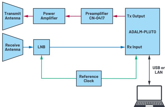
Figure 4. SDR satellite radio station.
