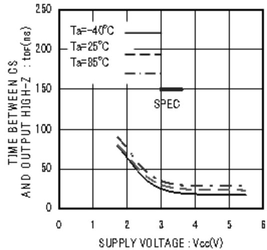
Figure 21. Time from CS to High-Z ttrf
