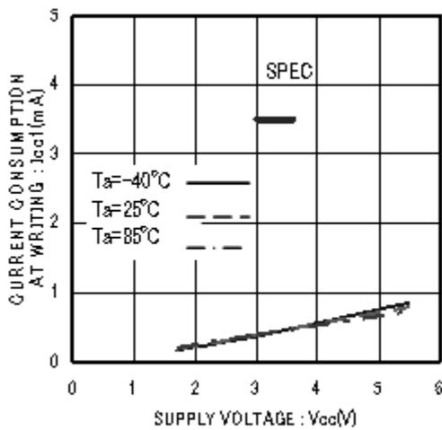
Figure 8. Current consumption at WRITE Action I<sub>cc1</sub>(fsk=2MHz)
