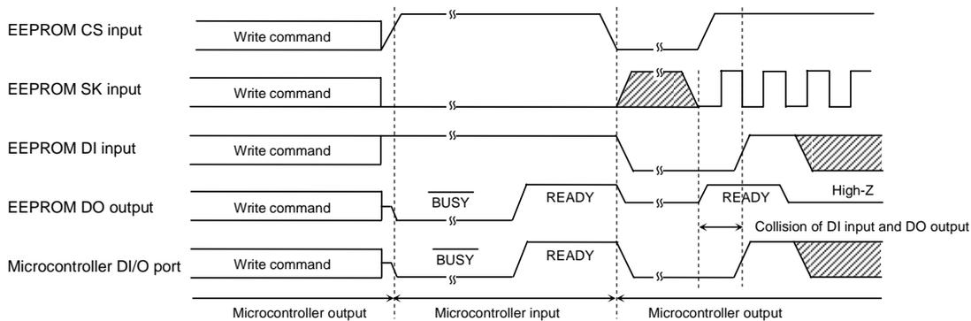
Figure 42. Collision timing at DI, DO direct connection
