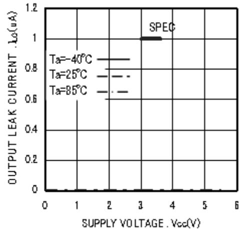
Figure 7. Output leak current I<sub>LO</sub>(DO)
