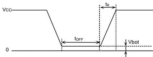
Recommended conditions of  $t_R$ ,  $t_{OFF}$ ,  $V_{bot}$
