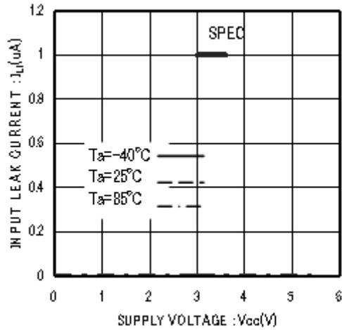
Figure 6. Input leak current I<sub>LI</sub>(CS,SK,DI)
