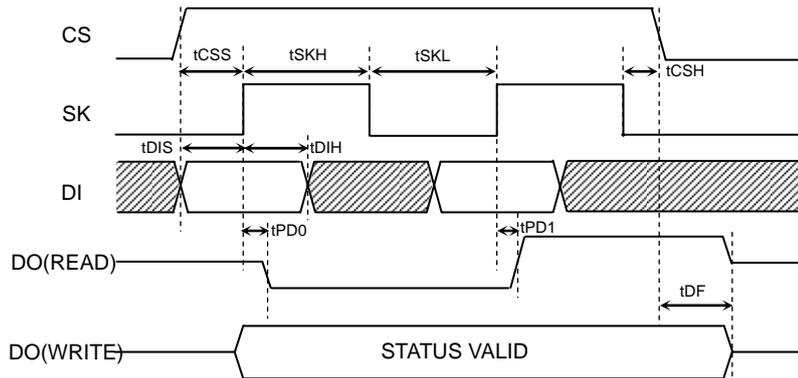
Figure 1. Sync data input / output timing
