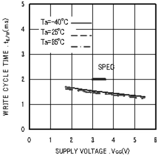
Figure 22. Write cycle time t<sub>EW</sub>
