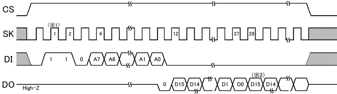
Figure 23. Read cycle (※2) Next address data (Auto increment function)
