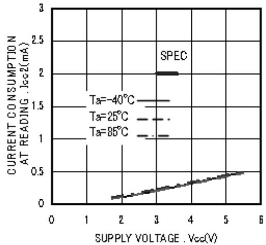
Figure 9. Consumption current at READ Action I<sub>cc2</sub>(fsk=2MHz)
