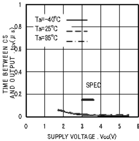
Figure 20. Time from CS to output establishment tsv
