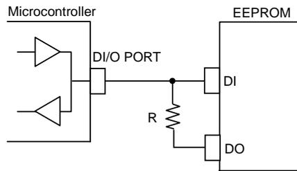
Figure 40. DI, DO control line common connection
