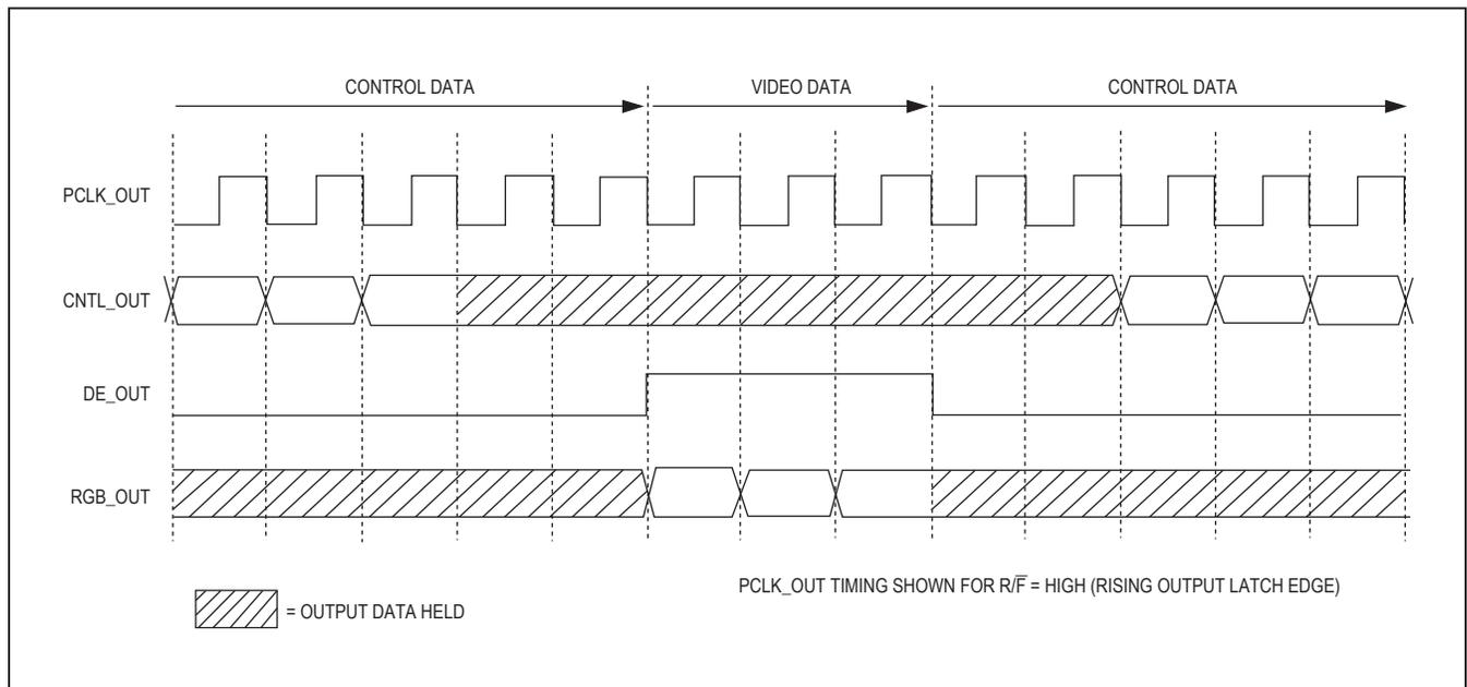
Figure 13. Output Timing
