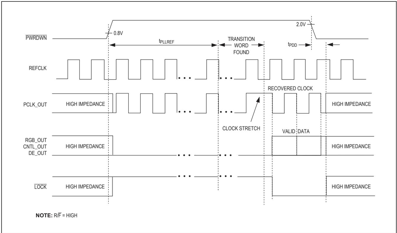
Figure 7. PLL Lock to REFCLK and Power-Down Delay
