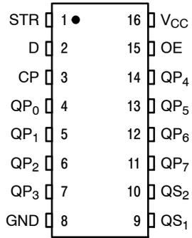
Figure 1. Pin Assignment
