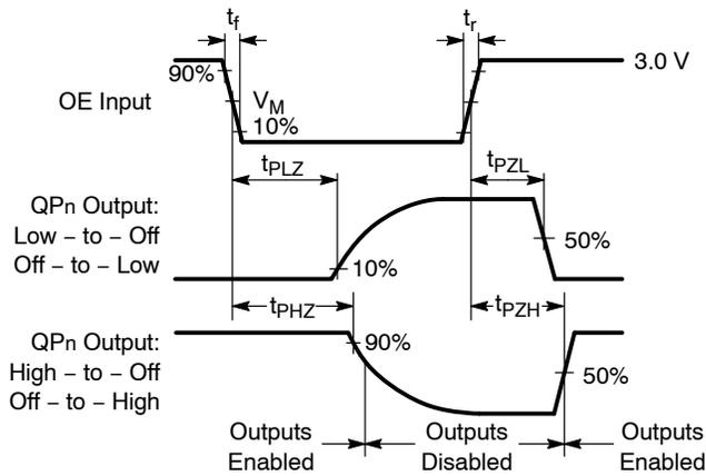
**Figure 9. Waveforms showing the 3-state enable and disable times for input OE.**
