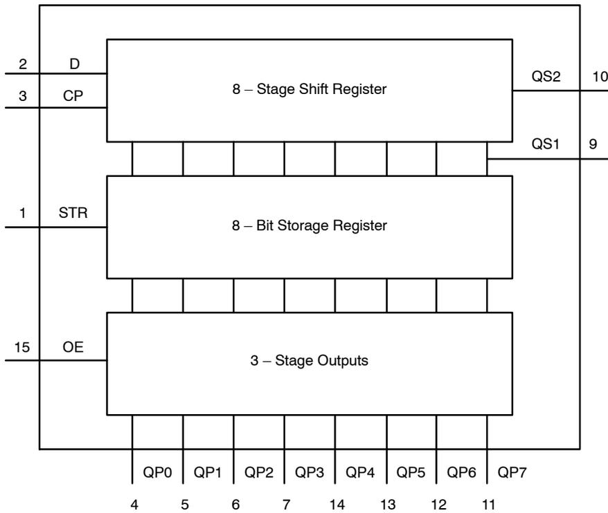
Figure 4. Functional Diagram
